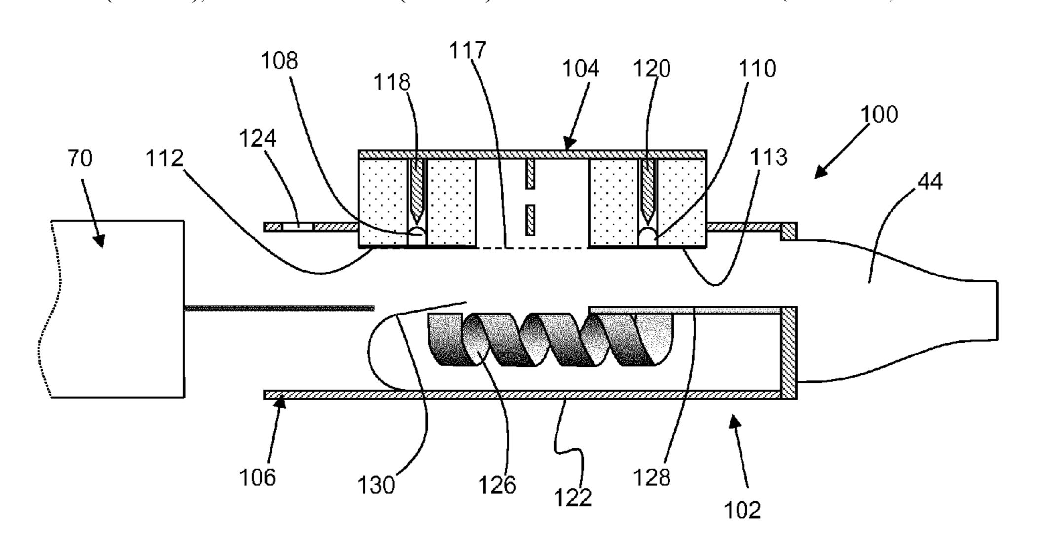
above a predetermined temperature results in displacement of the first end of the bimetallic strip away from the heater element.
