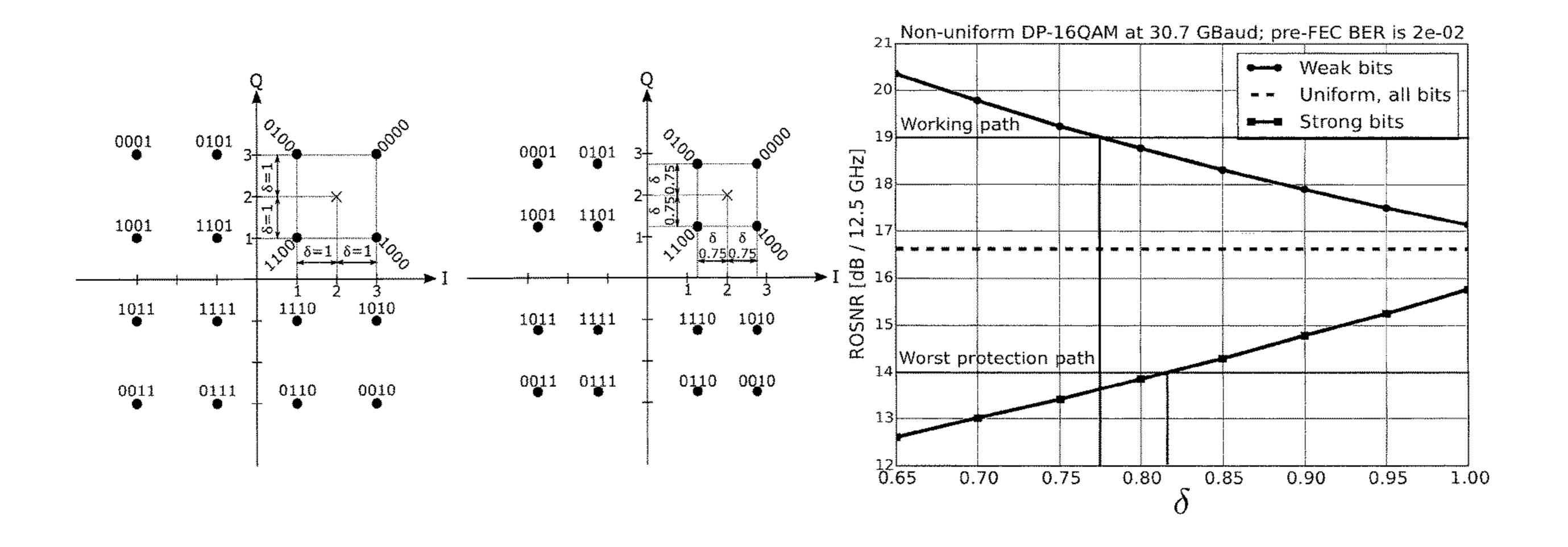
distortion such that a desired transmission quality for the transmission of the traffic of the highest priority class or classes via said predetermined protection link and a desired transmission quality for the full traffic via said given link are simultaneously ensured, and E) employing said distorted constellation diagram for transmission of digital data over said given link.
