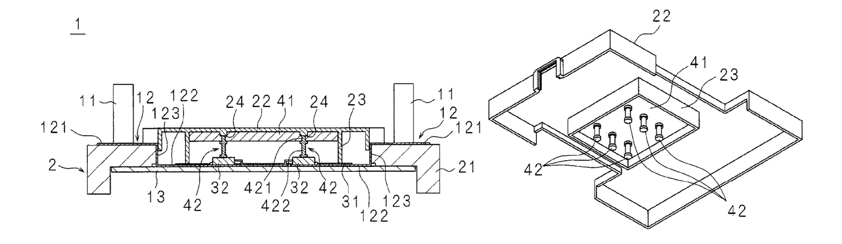
When the temperature of the switching element is low, the expansion material member is spaced apart from the circuit substrate and the switching element, and is disposed at a position opposing the one side. When the temperature of the switching element is high, the switching element is embedded in the thermally expanded expansion material member.
