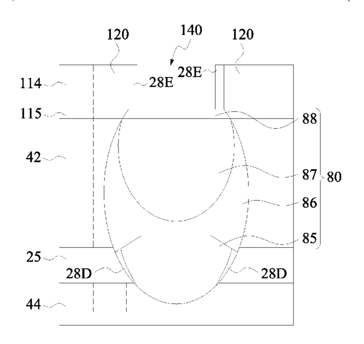
contact with the oxide layer and the stressor layer in the recessed portions.
