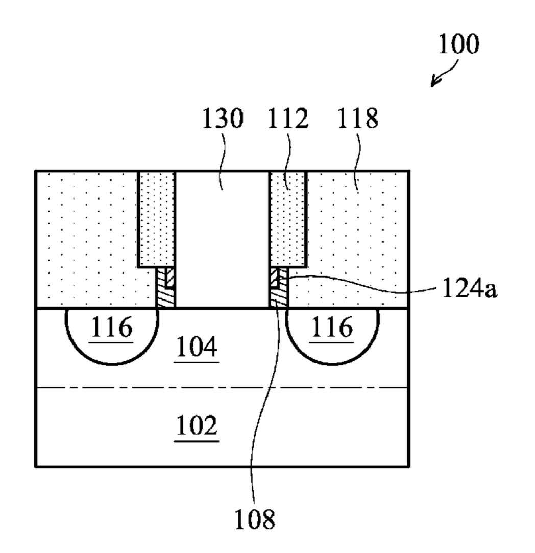
different materials, and wherein the second dielectric layer is in physical contact with the gate spacer and the first dielectric layer.
