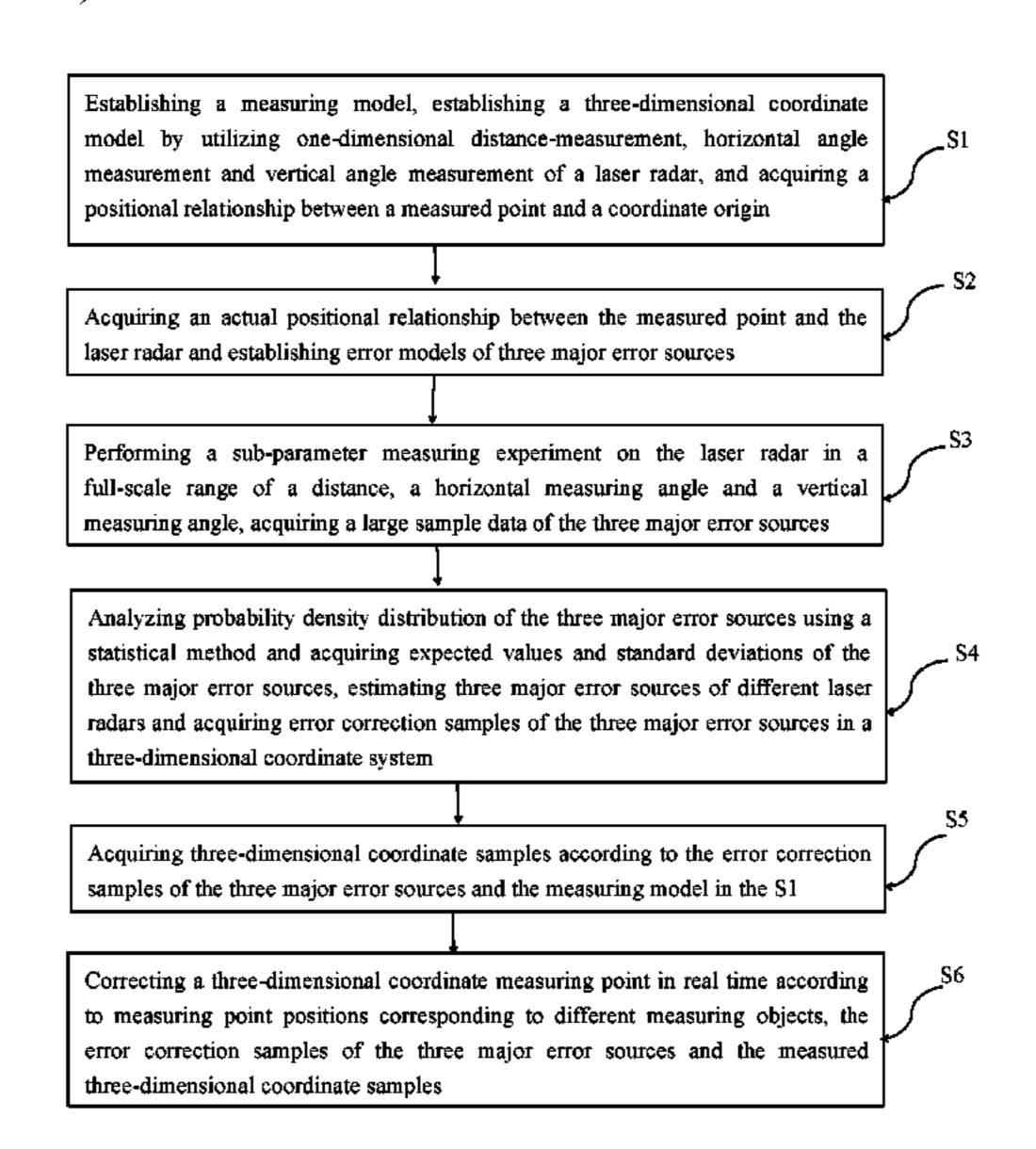
Establishing a measuring model, establishing a three-dimensional coordinate model by utilizing one-dimensional distance-measurement, horizontal angle measurement and vertical angle measurement of a laser radar, and acquiring a positional relationship between a measured point and a coordinate origin
