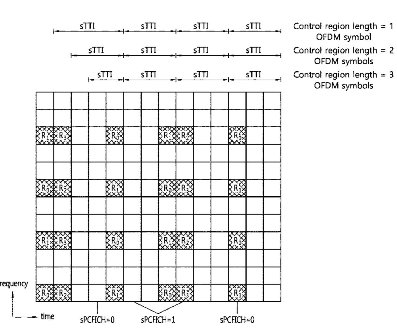
information included in a downlink control information (DCI) used for the second downlink channel and an RRC message. The control information and RRC message indicate frequency resources for the plurality of first downlink channels.
