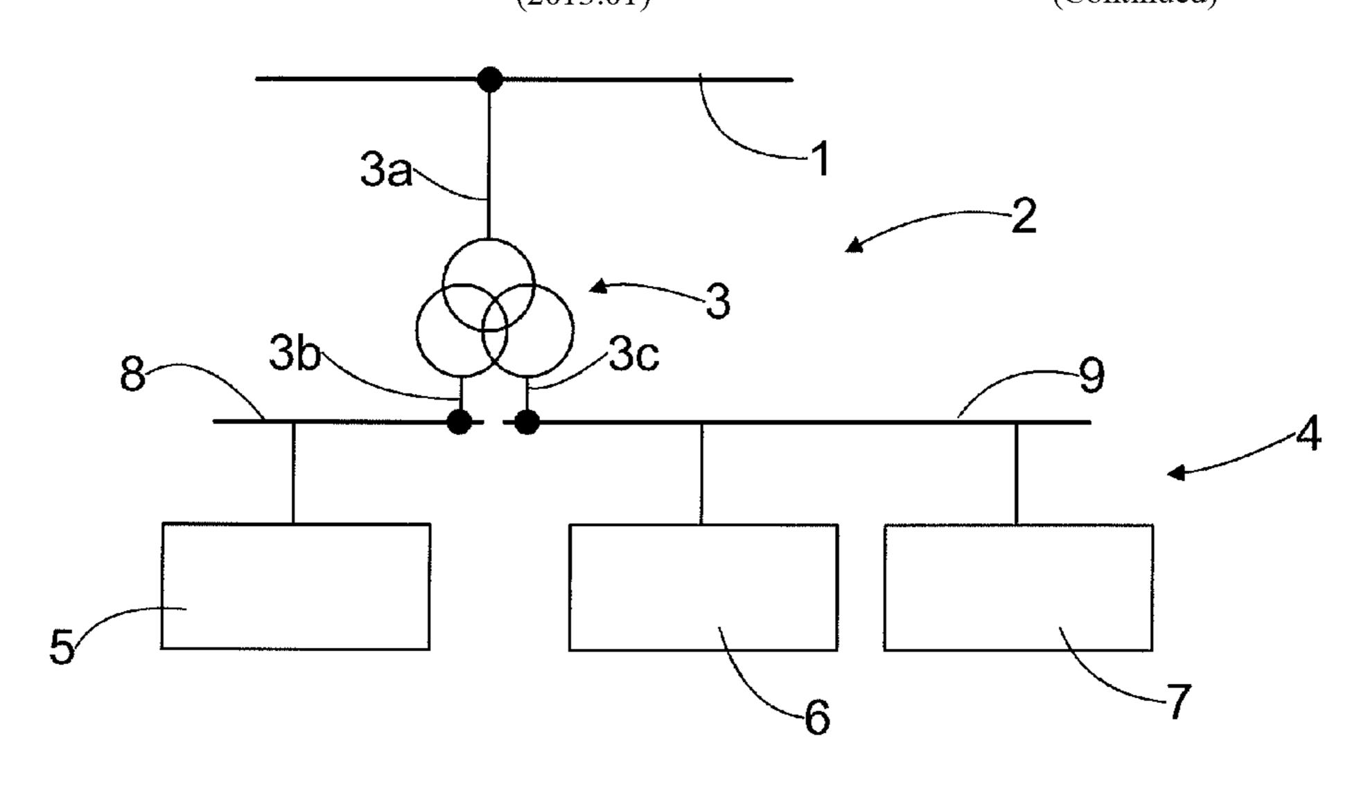
first low voltage side connected to the voltage source converter and a second low voltage side connected to the switched elements.
