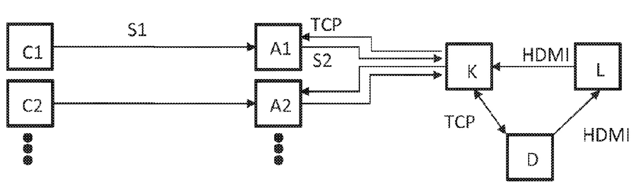
capturing device (C1, C2) is designed to capture the display information displayed on the display device (L), the analysis module (A1, A2) is additionally designed to ascertain quality data relating to the segmentation and transmit same to the control module (K), and the control module (K) is designed to adapt the display information displayed on the display device (L) on the basis of the quality data.
