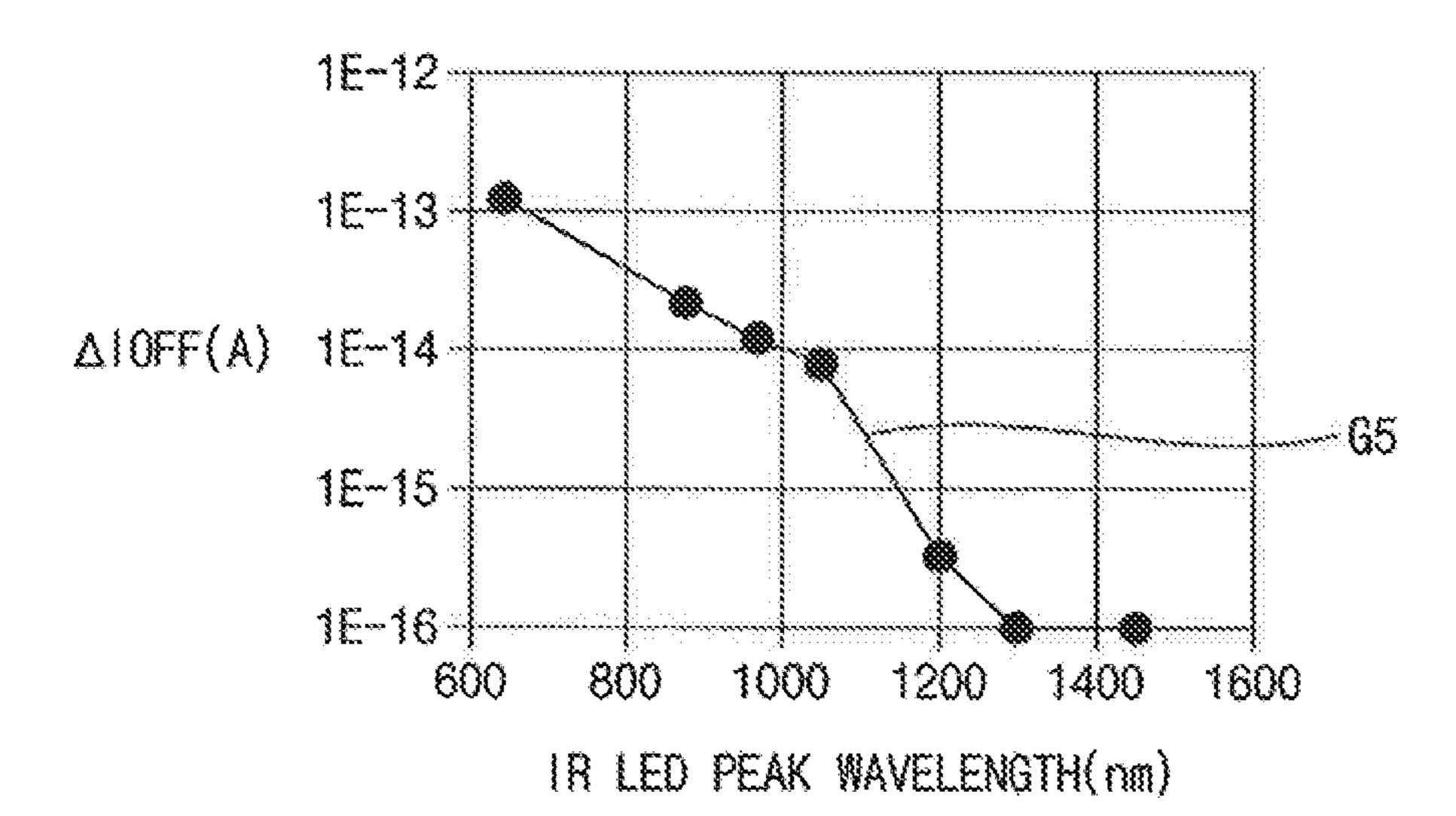
G5:CURRENT DIFFERENCE A 10FF BETWEEN FIRST LEAKAGE CURRENT AND SECOND LEAKAGE CURRENT
