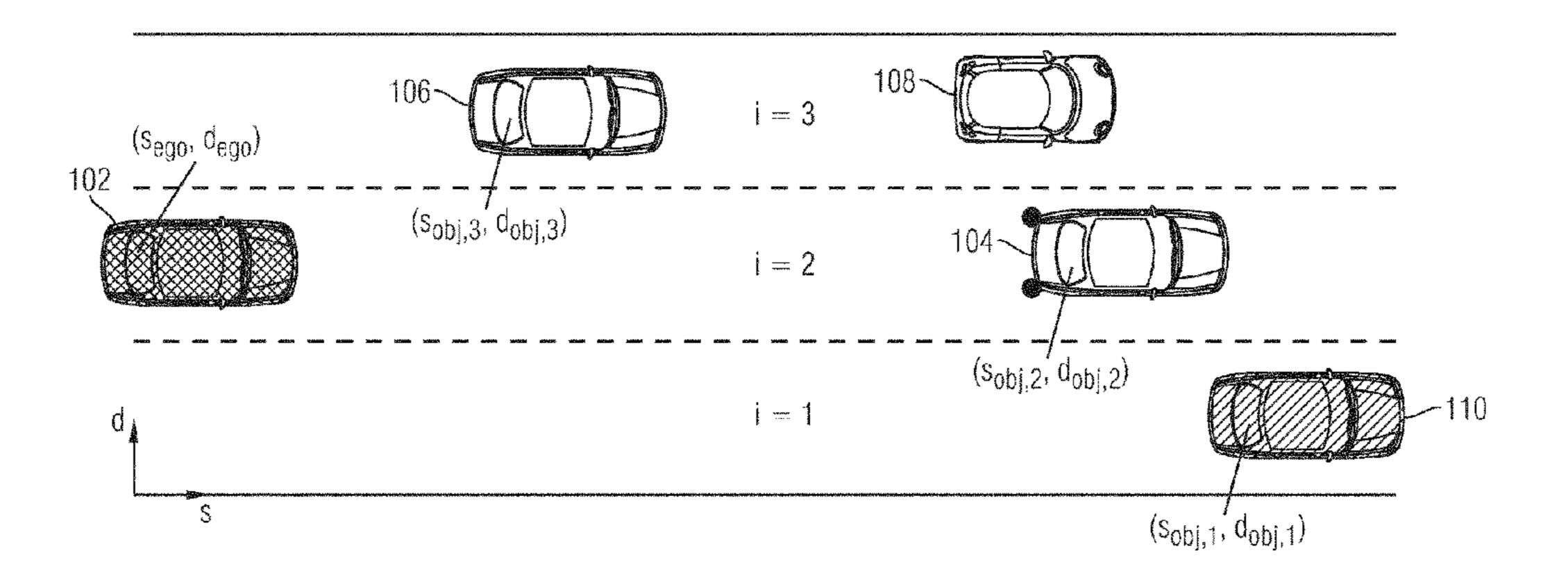
end time of the maneuvering process of the ego vehicle; and if the calculated distance of the ego-vehicle at the calculated end time of the maneuvering process equals a specified threshold or falls below a specified threshold: setting the specified speed of the object as the target speed of the ego-vehicle and transmitting the target speed to the trajectory planning process in order to calculate a following trajectory for the ego-vehicle.
