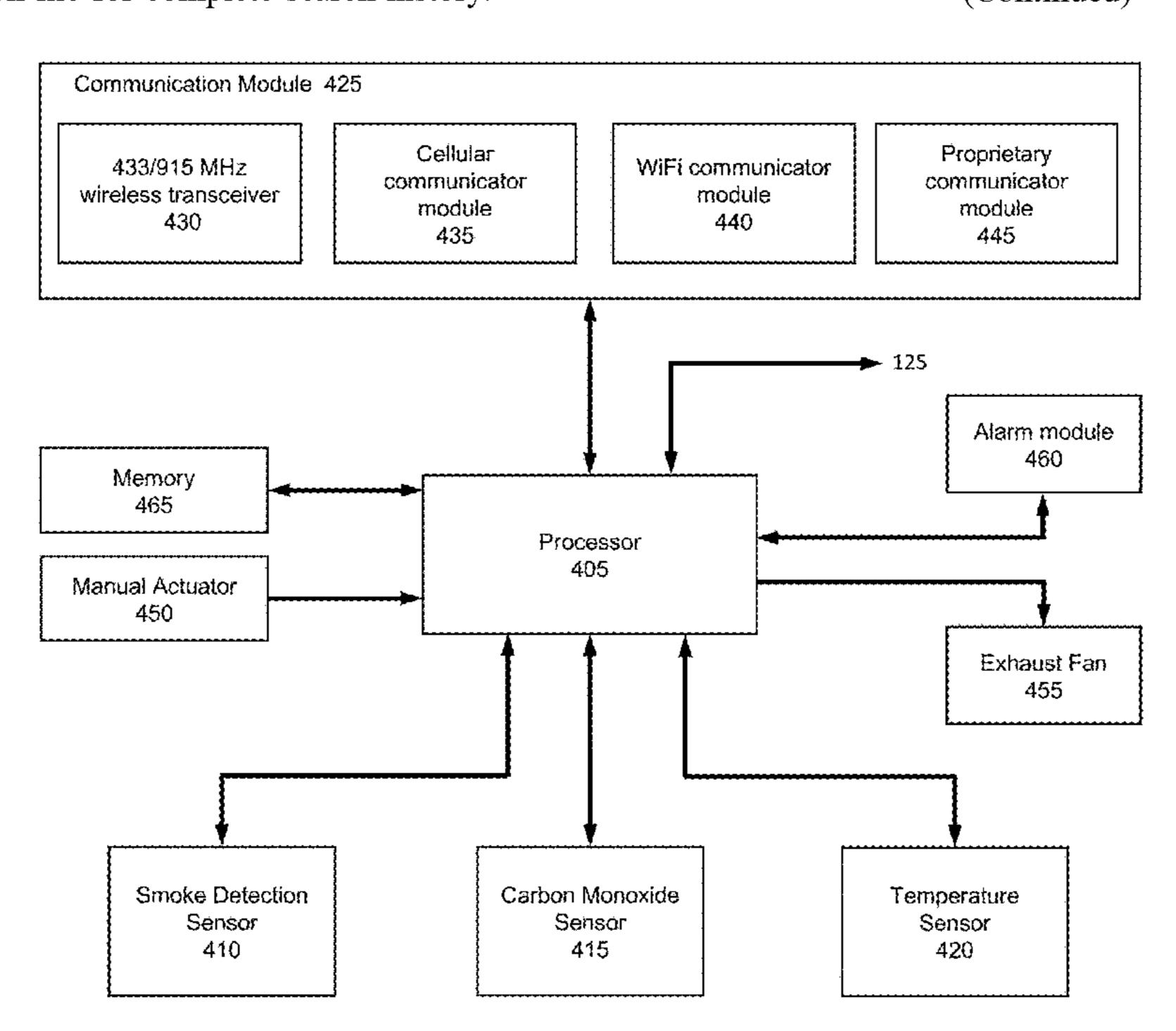
the alarm module when the detected measure is above the predetermined threshold and generates a message to be wirelessly communicated to the monitoring central station by the communication module, the message including the detected measure and a unique identifier of the detector.
