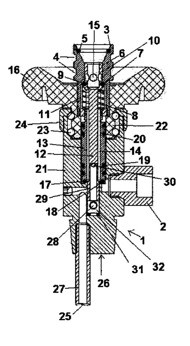
opening at the bottom side can be connected to the gas tap in a gas-conducting manner, specifically typically by rotating a corresponding rotary handle. The hose-shaped or tubular line protrudes relative to the opening, specifically in particular by at least by 200 mm, particularly preferred by at least 300 mm. A method concerns the refilling of a liquid gas bottle comprising the claimed fitting.
