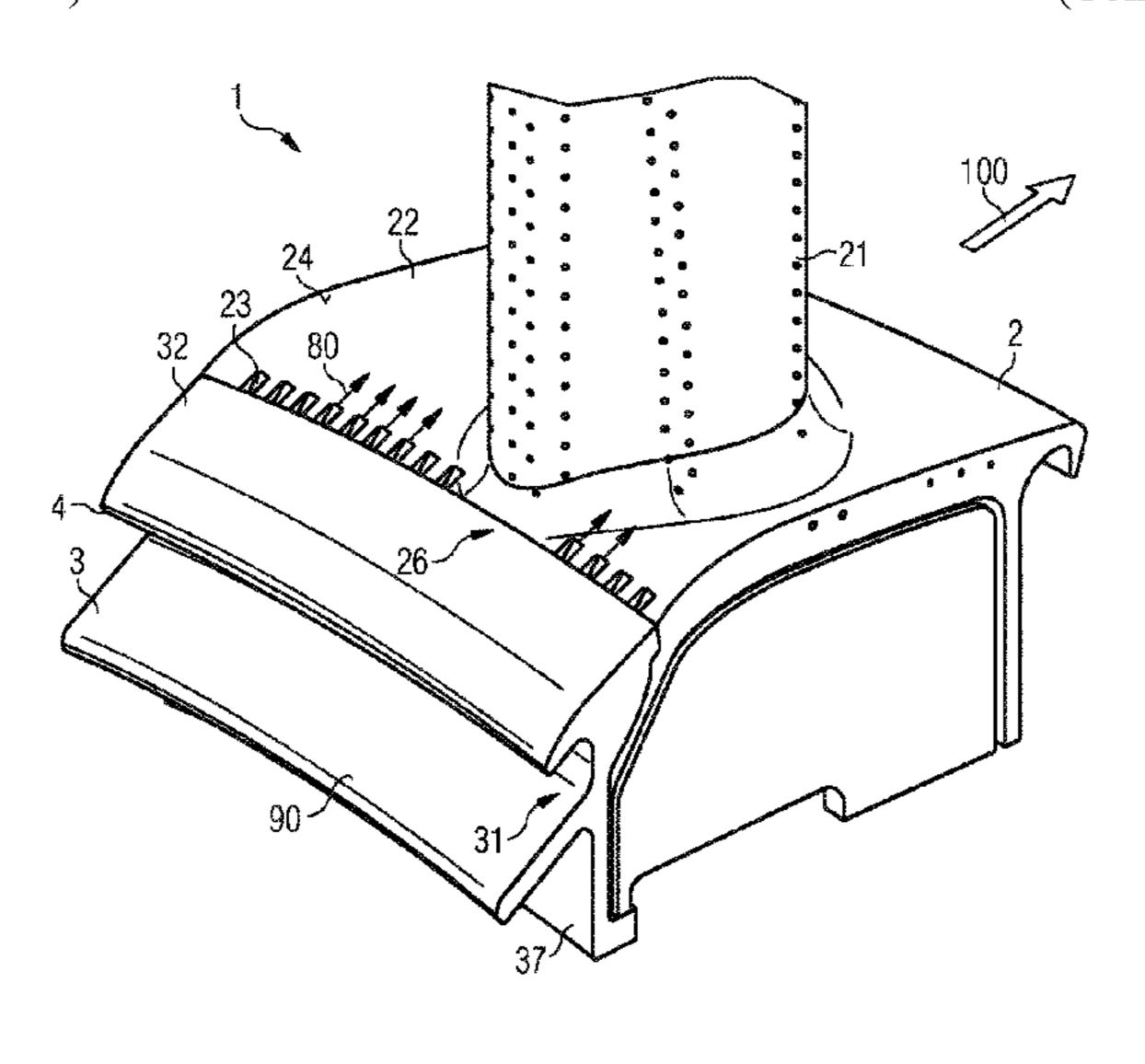
the first platform section for film cooling of the surface, the slots being provided at an upstream bend of the first platform section and the slots are provided on a side of the first platform section facing the working fluid.
