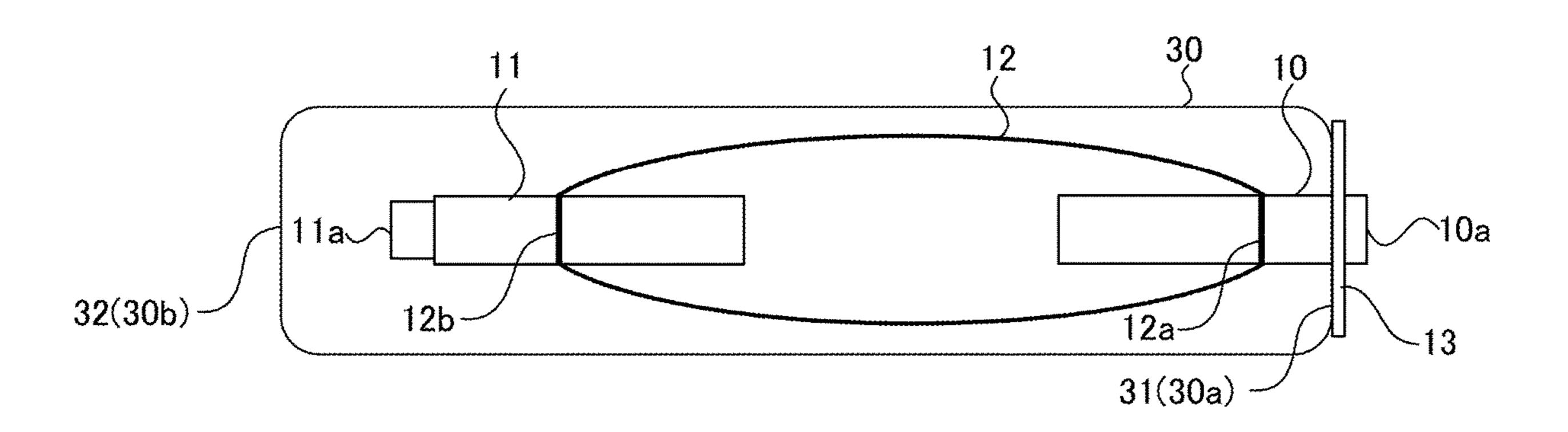
liquid supply apparatus includes a first support member, a second support member, a balloon having one end supported by the first support member and the other end supported by the second support member, and a casing having a constant longitudinal length. The balloon is disposed in the casing and is configured so as to be able to hold a liquid therein and discharge the liquid therefrom. When the balloon holds the liquid, the one end and the other end of the balloon are positioned in the case.
