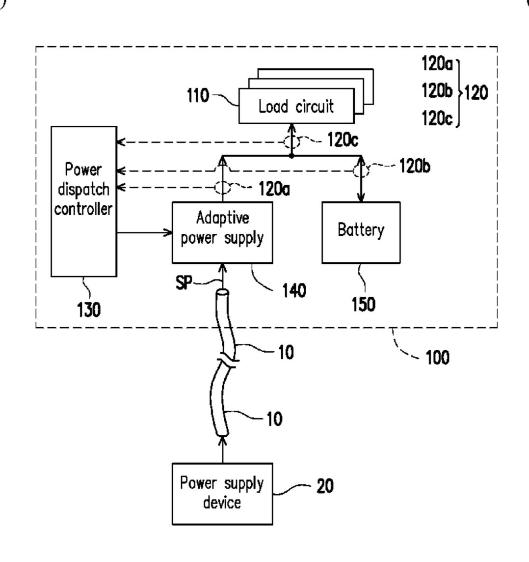
power supply and the battery power the load circuit by adjusting the output of the adaptive power supply.
