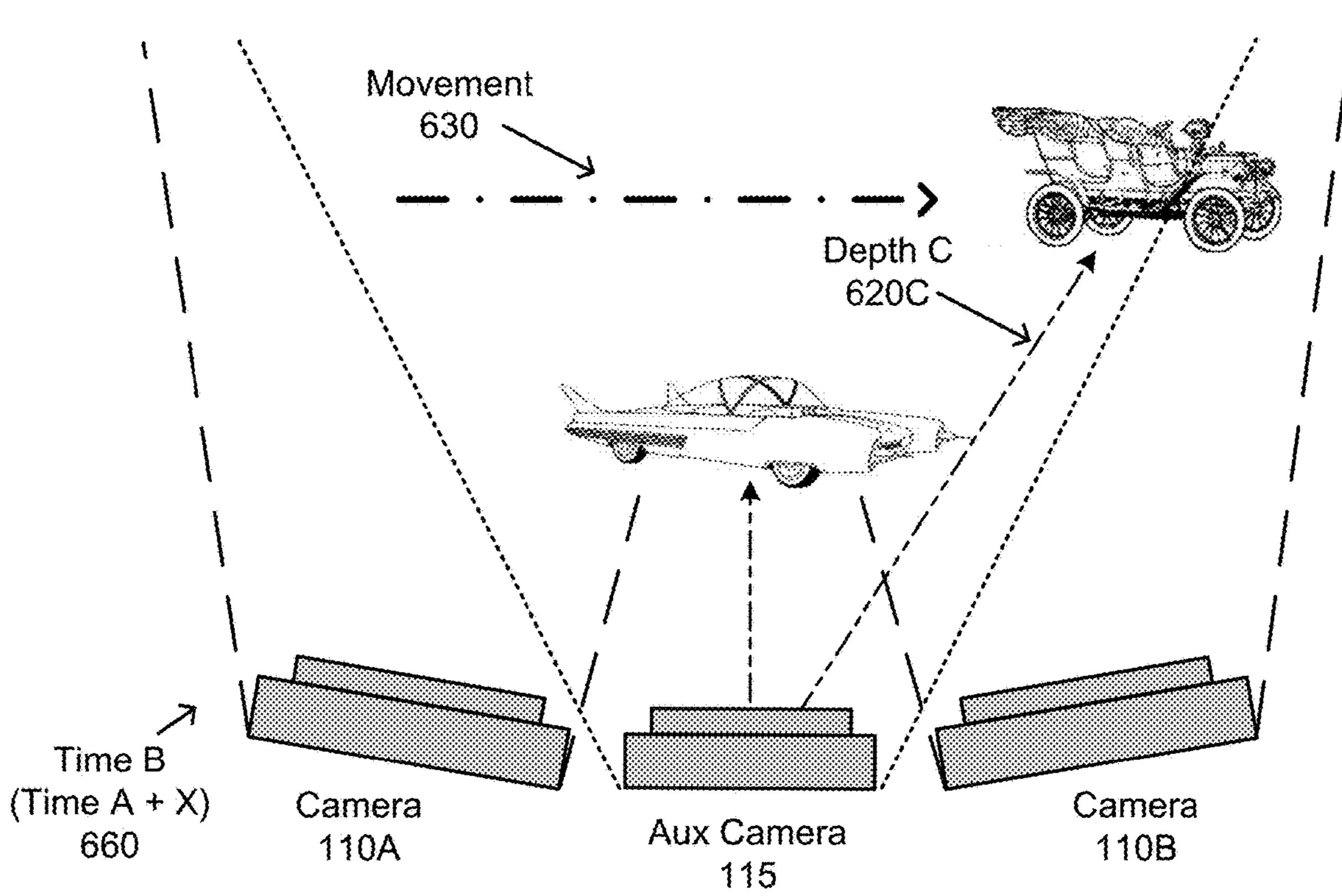
Capture a set of four images from an array of four cameras, each camera of the array of four cameras having an overlapping field of view (FOV) with an adjacent camera of the array of four cameras.
