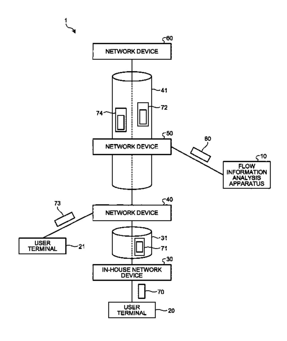
sis apparatus extracts information on the header of the IP packet from the header sample on the basis of a result of a search through the header sample for a byte sequence that matches search data in which a value that is set in a specific field of the tunnel header and a value that is set in a specific field of the IP packet are combined.
