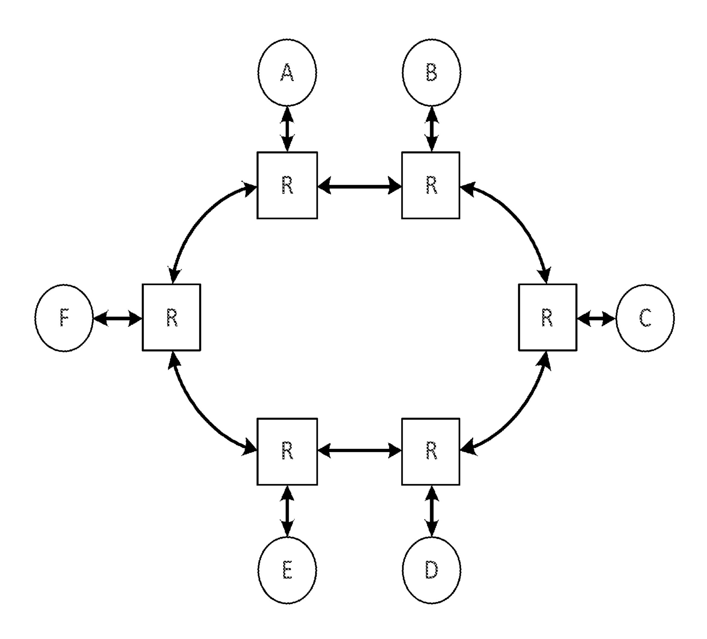
a Bi-directional ring topology utilizing router(s) {R}
