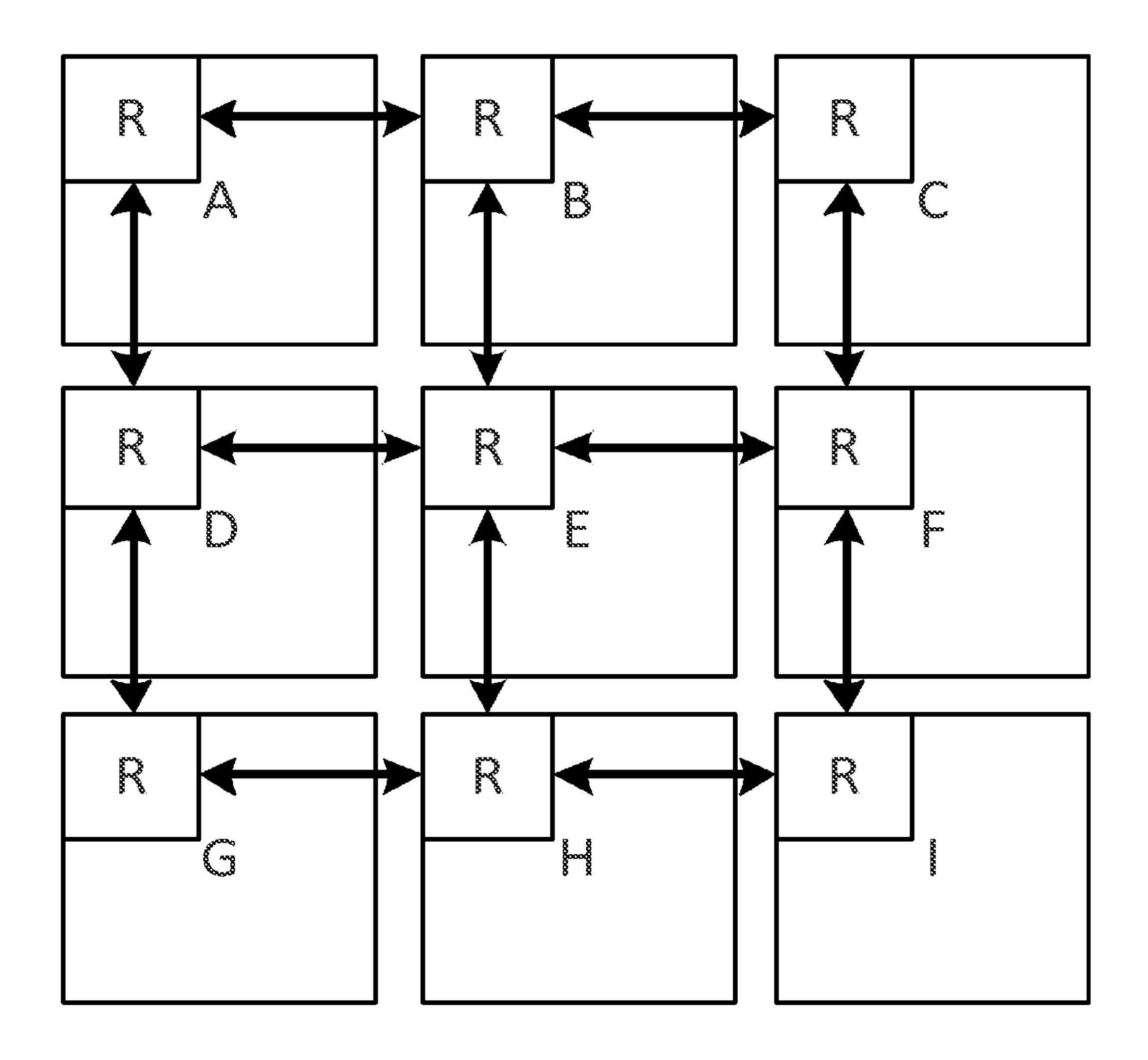
a 2D Mesh topology utilizing router(s) {R}
