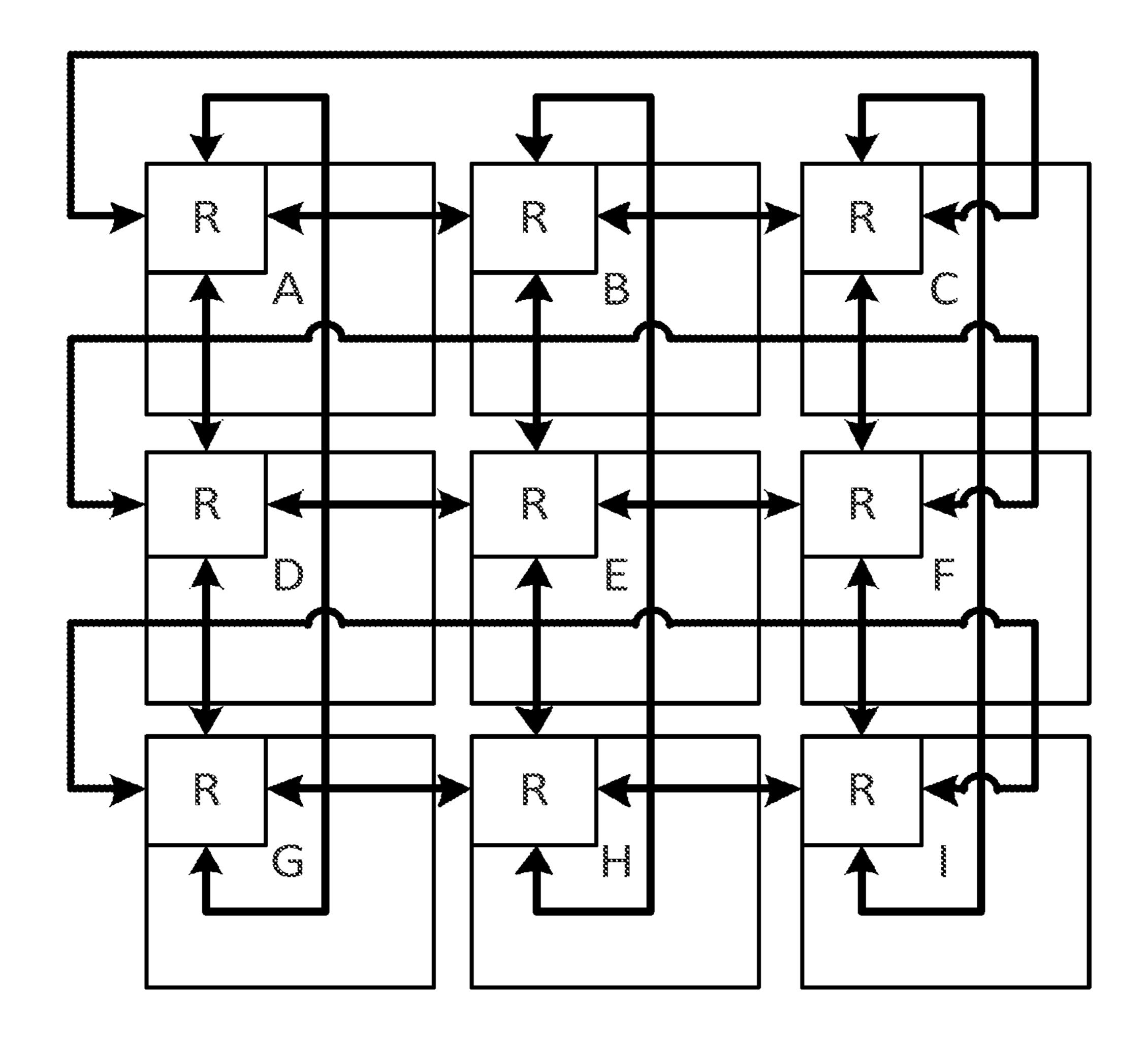
a 2D Taurus topology utilizing router(s) {R} FIG. 1(c)
