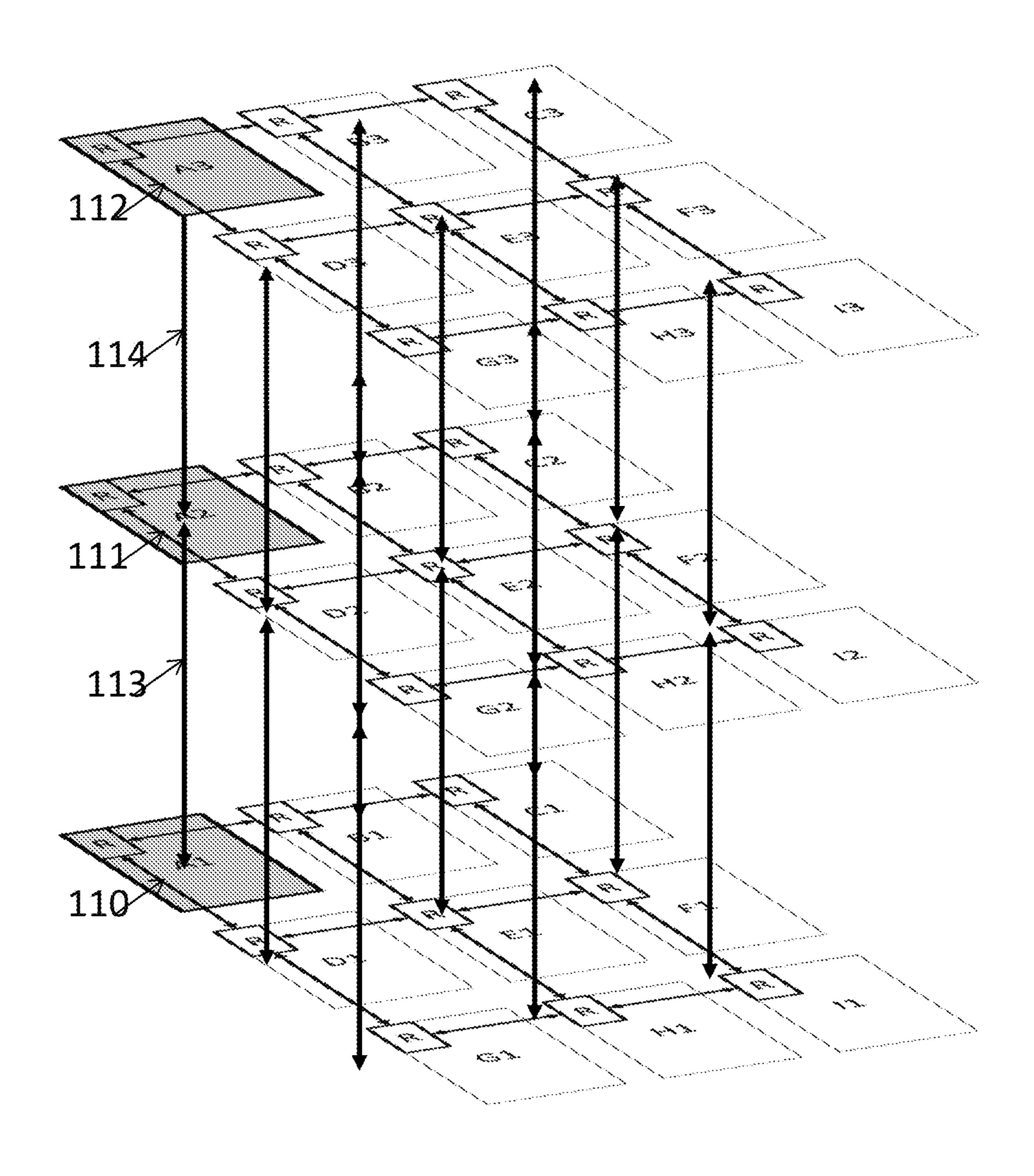
a 3D Mesh NoC topology utilizing router(s) {R}
