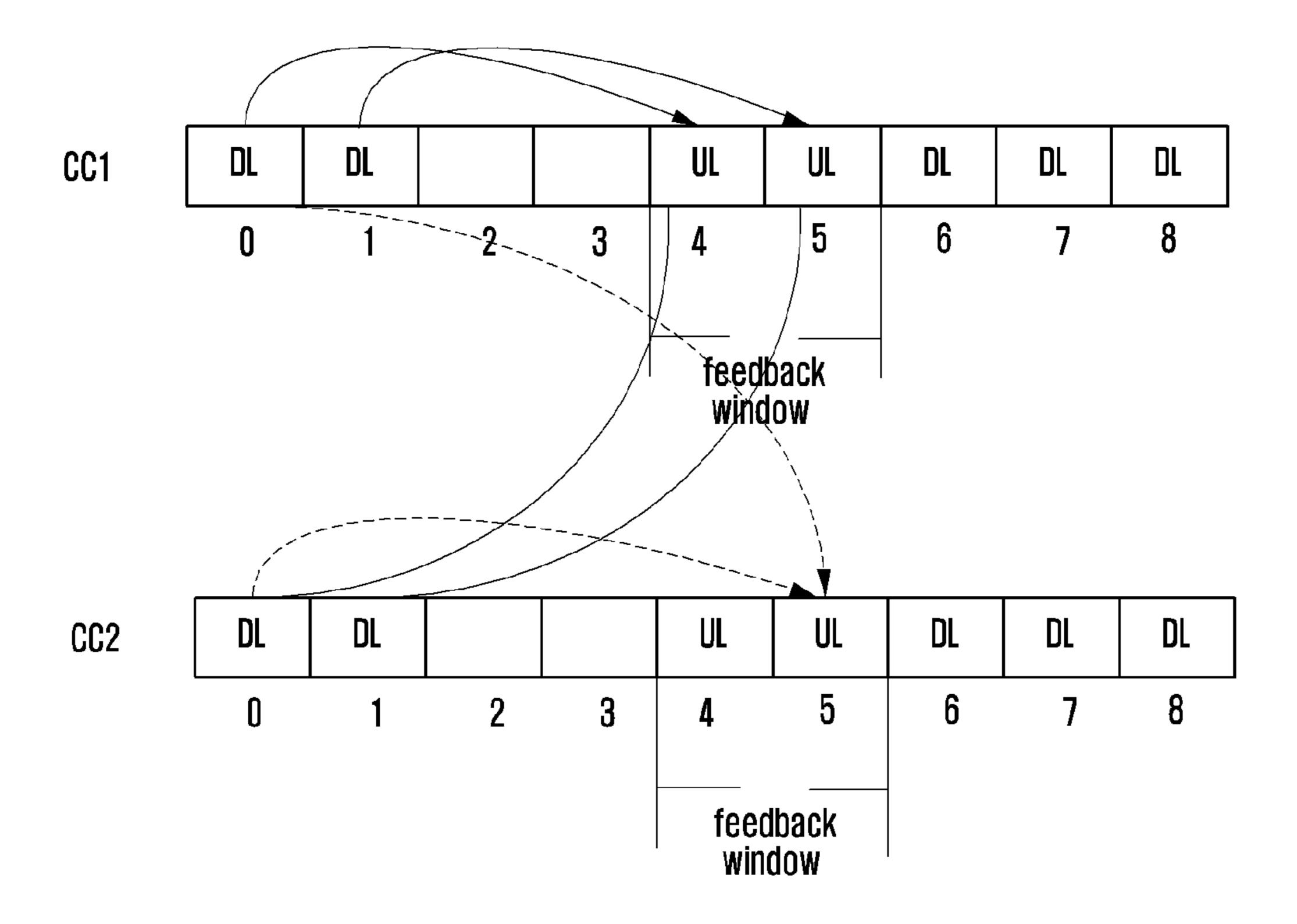
a UE determines an uplink subframe n+k for HARQ-ACK feedback of PDSCH(s) in a downlink subframe n, and determines whether periodic CSI needs to be fed back in uplink subframe n+k
