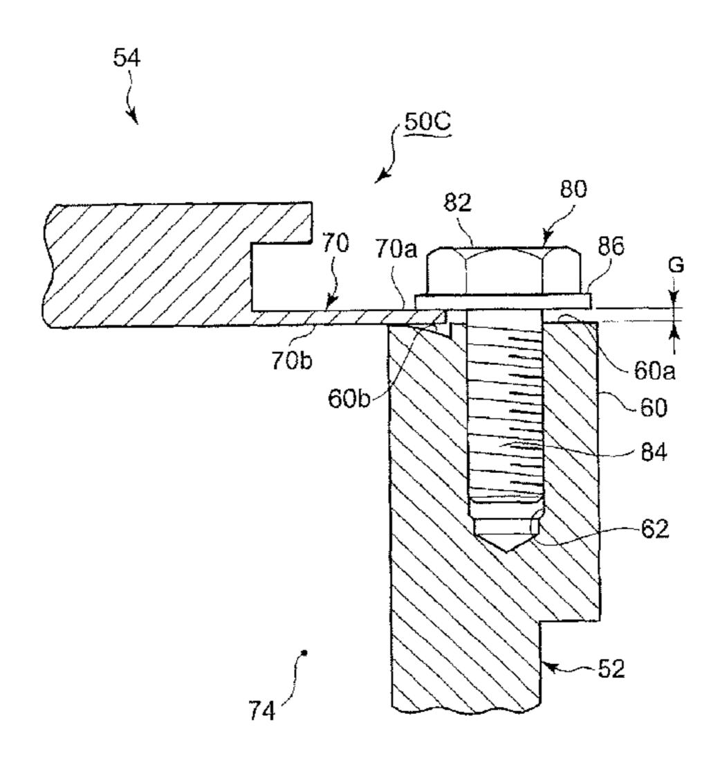
surfaces 44a make tight contact with the outer end face 60a so as to resiliently deform the sealing ring 48.
