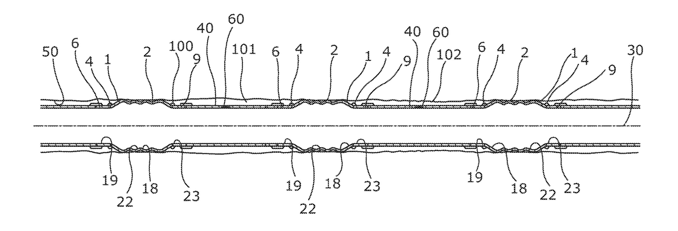
metal structure having a plurality of tubular sections and at least one annular barrier according to the present invention, and to a completion method of preparing an annular barrier according to the present invention.
