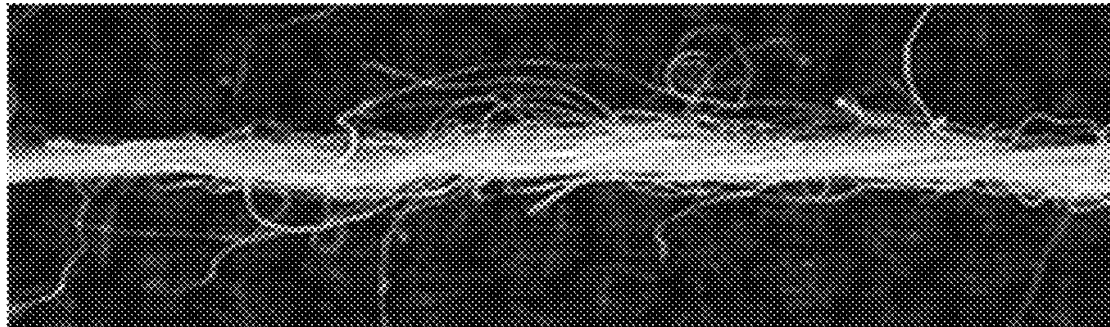
(a) Hemp-blended single spun yarn produced by a conventional method
