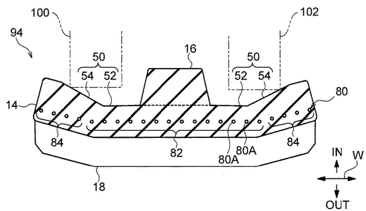
represented by L, then a result of subtracting a turning direction length of the crawler main body at the flat portion (72) from a turning direction length of the crawler main body at the slanting portion (74) is less than  $2\pi L$ .
