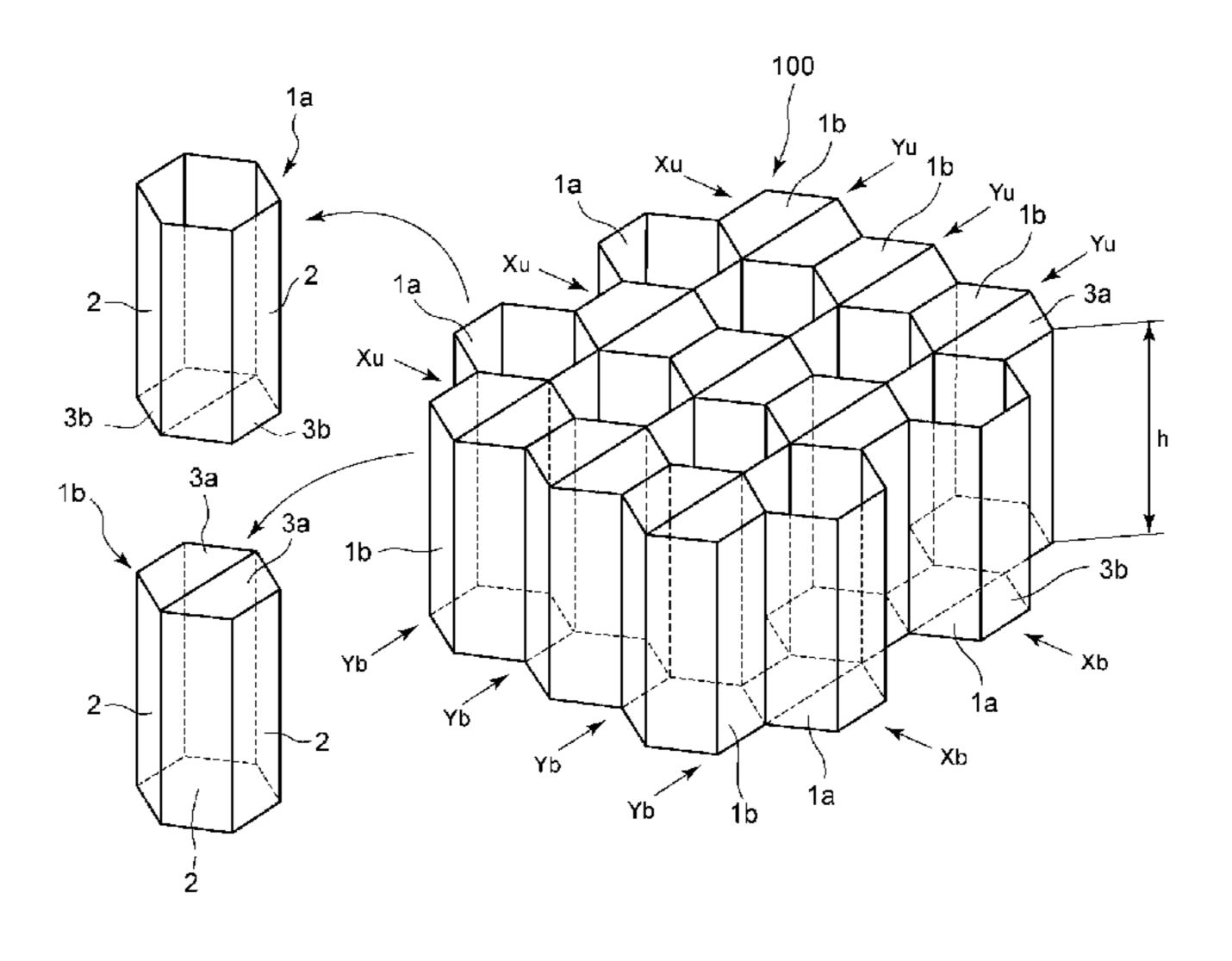
amide (A):aliphatic polyamide (B) is within a range of 100:25 to 400 by mass standard. Also provided is a sandwich structure obtained by disposing flat plates at the top surface and bottom surface of the honeycomb structure, and a honeycomb substrate obtained by molding the thermoplastic resin composition into a film or a sheet.
