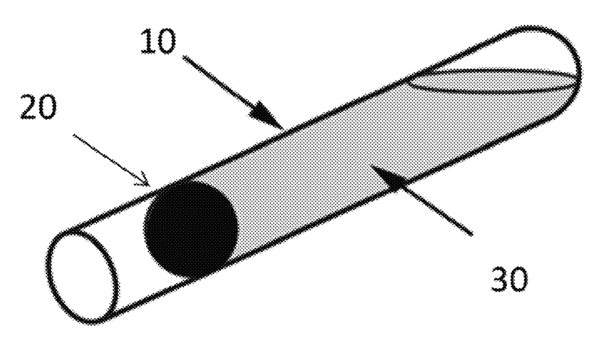
biodegradable cylindrical container with one open end. The open end will be plugged with a piece of water absorbent polymer or gel, for example, polyacrylamide gel, sodium alginate. The water absorbent polymer or gel absorbs the liquid bait and expands inside of the cylindrical container so that it will function as a polymer "wick" to deliver a small amount of the liquid bait to foraging ants.
