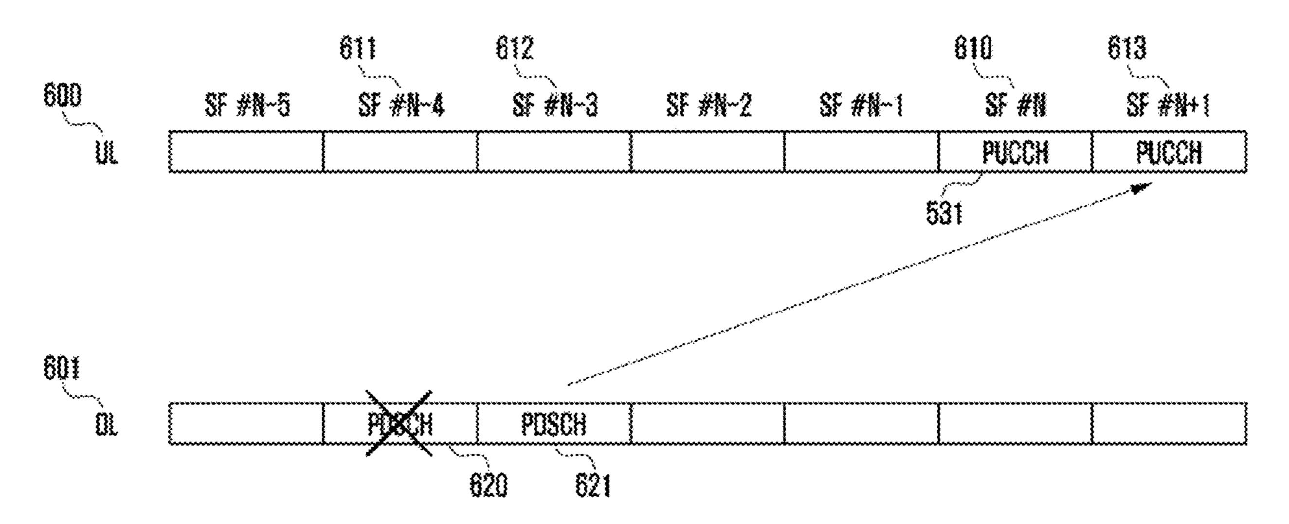
whether an uplink resource where the ACK or NACK information is received is included in a first resource or a second resource; and interpreting, in particular by the base station, the ACK or NACK information as ACK if the uplink resource where the ACK or NACK information is received is included in the first resource.
