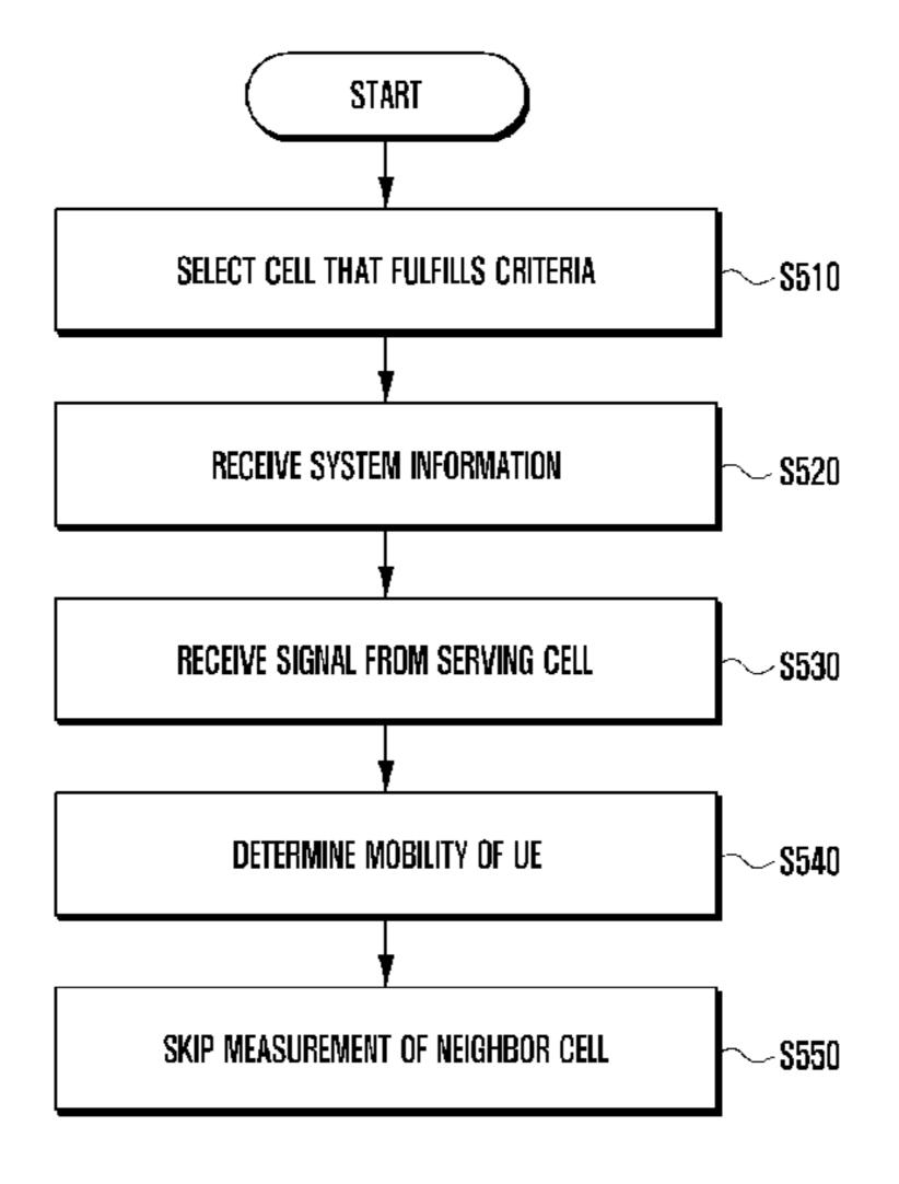
and an IoT related technology. A method for a terminal according to the present invention comprises the steps of: receiving system information; receiving a signal from a service cell when a discontinuous reception (DRX) timer expires; determining the mobility of the terminal on the basis of the signal; and omitting neighboring cell measurement when the terminal has no mobility.
