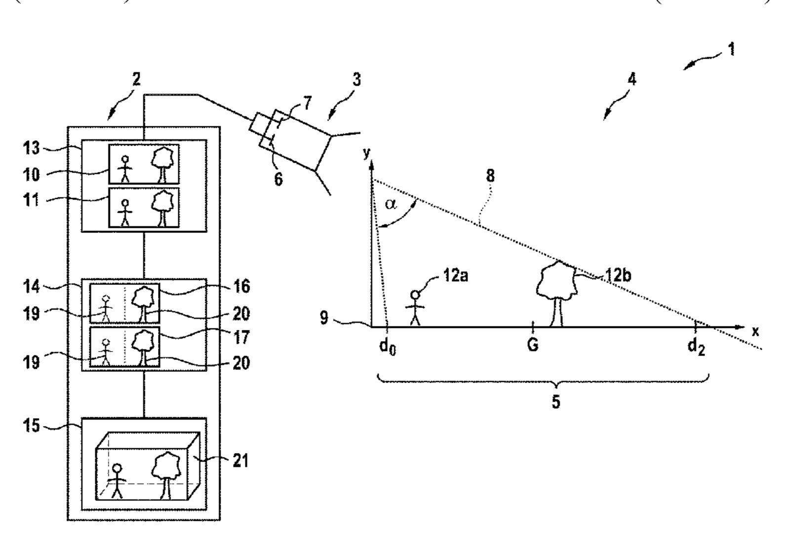
used to stereoscopically evaluate the monitoring area (5) based on the first reduced image (16) and the second reduced image (17).
