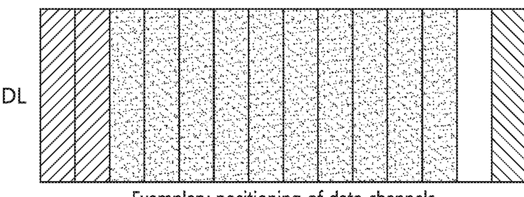
Exemplary positioning of data channels during downlink transmission
