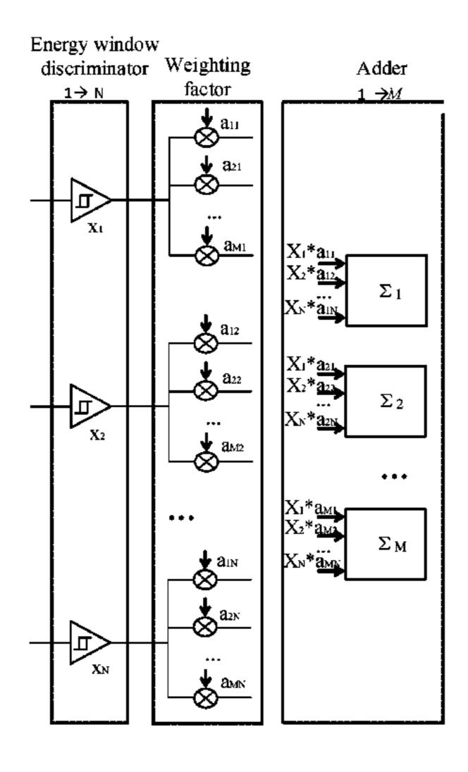
M is an integer greater than 0; and obtaining output results of the M output channels based on the weighting factor matrix and numbers of photons having an energy range falling into individual energy windows of the number N of energy windows.
