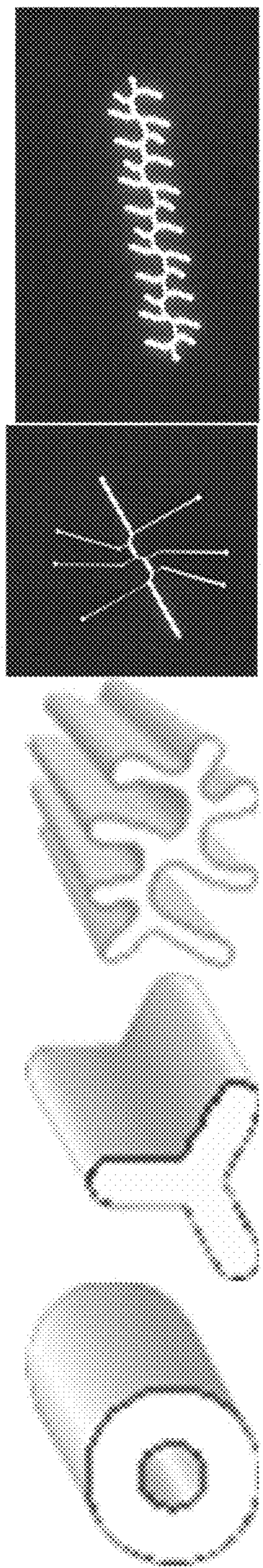
Hollow Trilobal Octalobal Starfish Caterpillar
