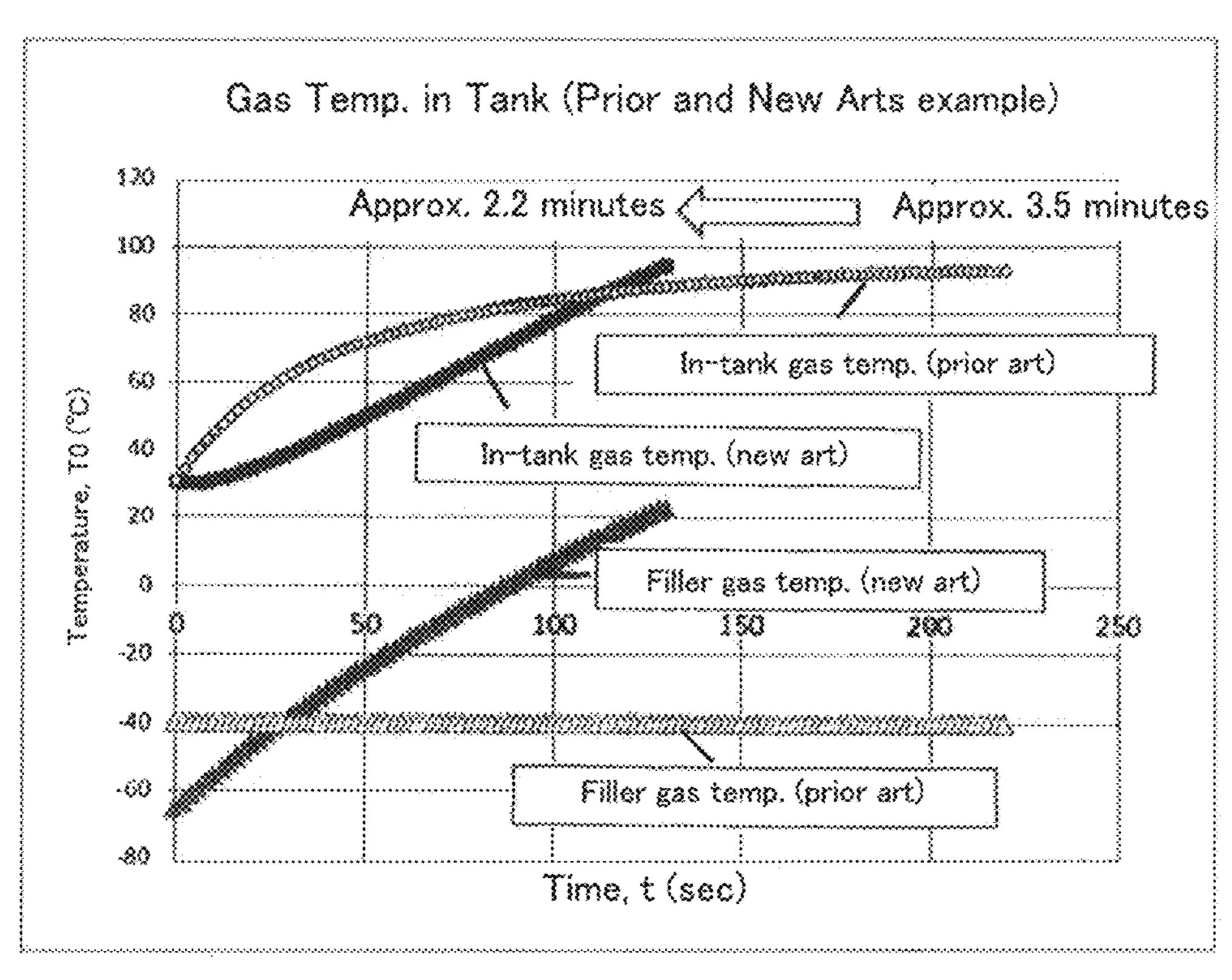
Tank capacity:156L Hydrogen gas source pressure:82MPa (A) Temperature:30°C Initial tank pressure:8MPa (A) Initial tank temperature:30°C
