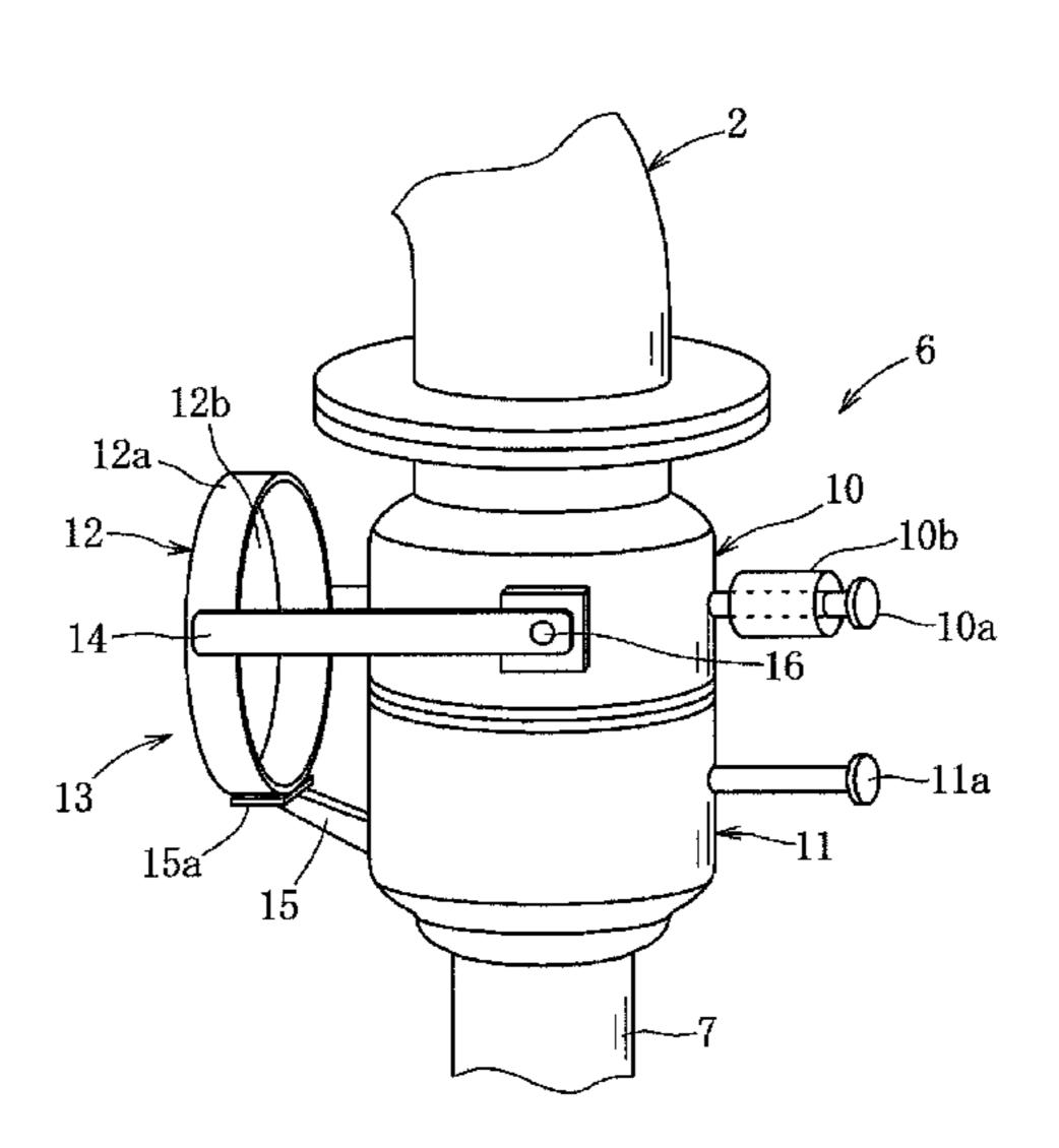
unit is separated from the first shut-off valve unit, and the system includes a container support mechanism which is capable of retaining the reservoir container at a retracted position in a state in which the first and second shut-off valve units are connected to each other, the container support mechanism being configured to automatically shift the reservoir container to a reserving position, in a state in which the first and second shut-off valve units are separated from each other.
