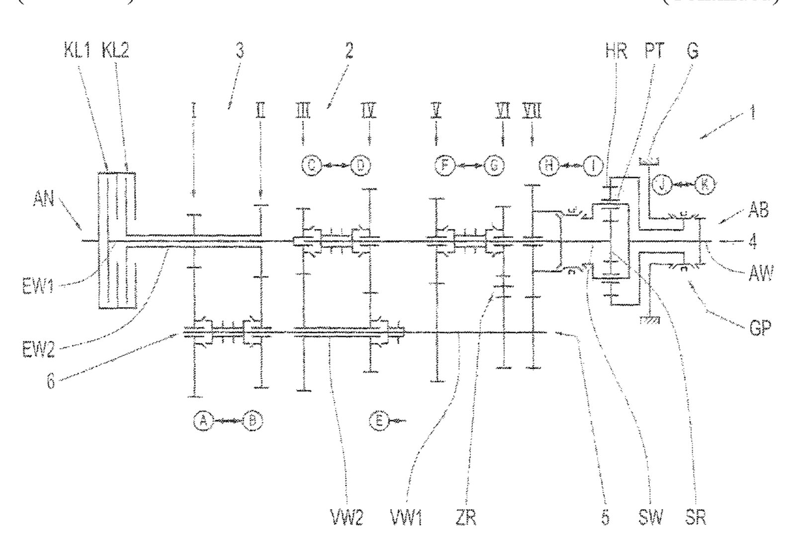
ments are connected to the second countershaft. Opposite sides of the intermediate shaft are respectively connected to a range group and the output shaft.
