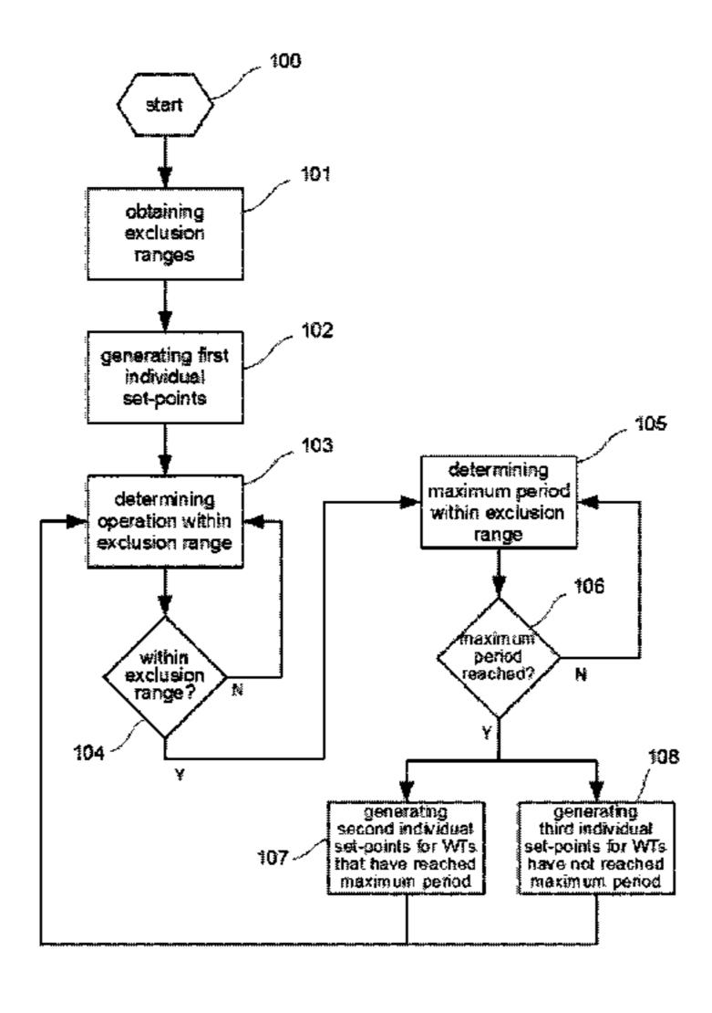
turbines to cause the set of wind turbines to generate the total active power. Systems suitable for such methods are also provided.
