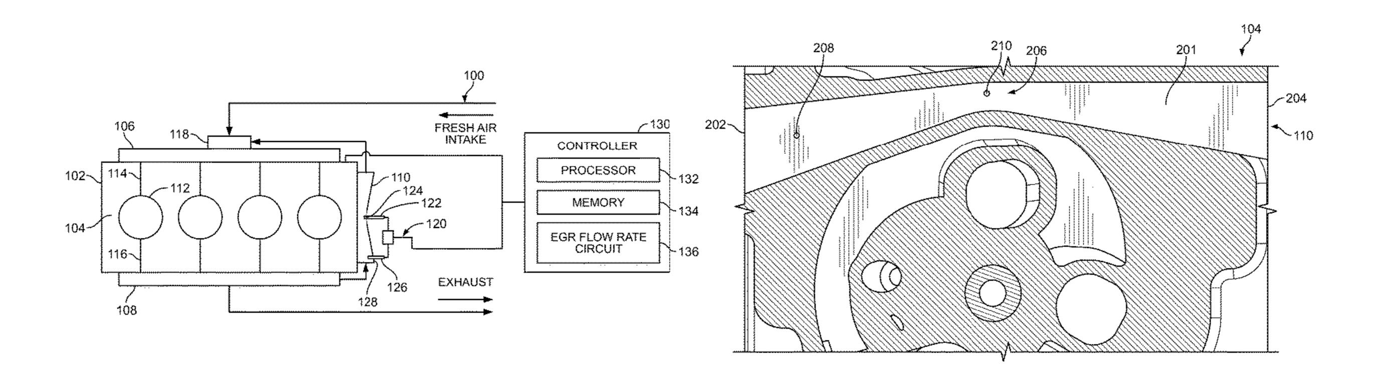
port is positioned proximate the first end. A differential pressure sensor includes a first pressure sensor positioned in the first sensor port and a second pressure sensor positioned in the second sensor port.
