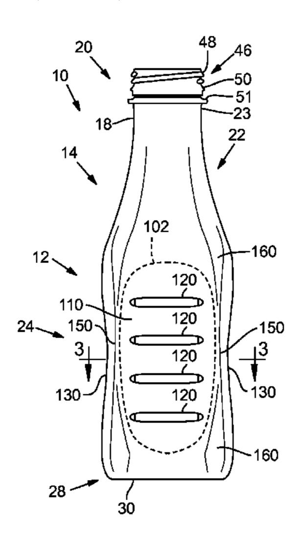
the label boundary panel and bound thereby. The inwardly-directed rib(s) generally aid(s) the label boundary panel to resist the vacuum force.
