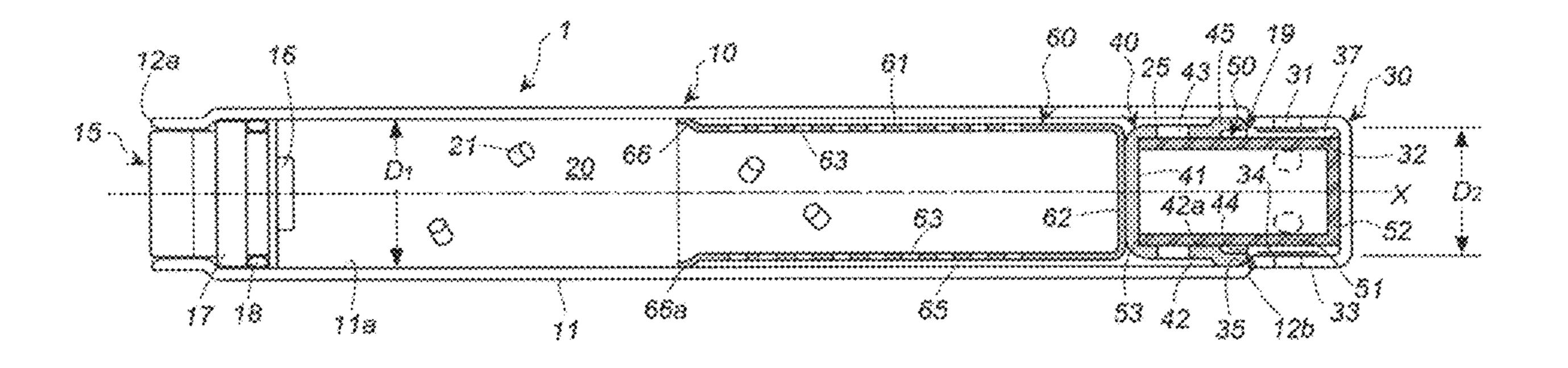
a filter disposed in a space surrounded by the cup-shaped member and the diffuser portion,
