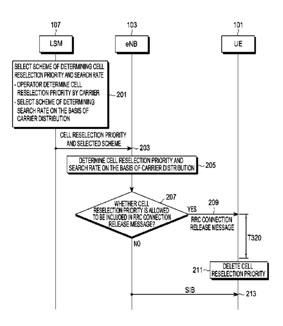
basis of the determined search rate, and a process of transmitting the determined cell reselection priority to the idle UE.
