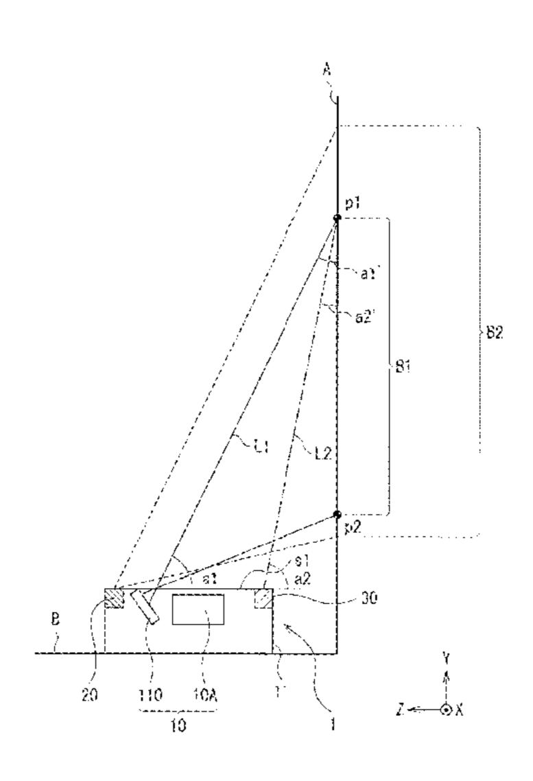
imaging unit. The imaging unit performs capturing of the linear light with which the projection surface is irradiated, and the signal processor corrects, on a basis of a captured image of the linear light, a distortion of the projected image.
