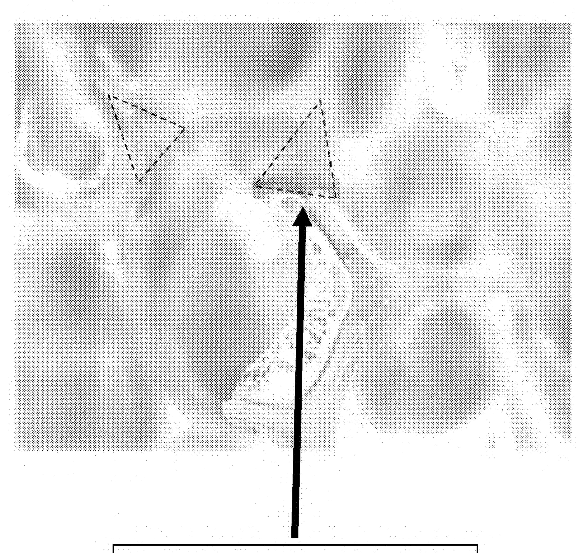
W = the average of the length of each side of the measured triangular area is set as the width W of the nodal section of the foam cell wall surface of an elastic layer.
