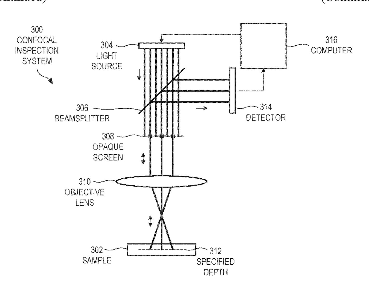
collected light, for example, by directing the collected light onto a single-pixel detector, or by directing the collected light onto a multi-pixel detector and averaging the pixel output signals to form a single electronic signal. Averaging the incident and/or return light can be advantageous for structured or inhomogeneous samples.
