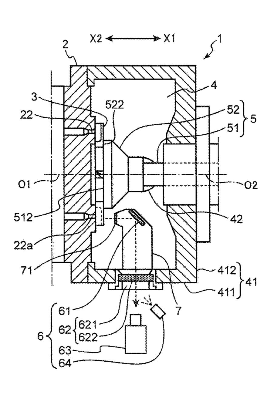
the inside of the housing chamber to the outside of the housing chamber. Thus, with this pelletizer apparatus, the cut section can be visually checked clearly via the optical system.
