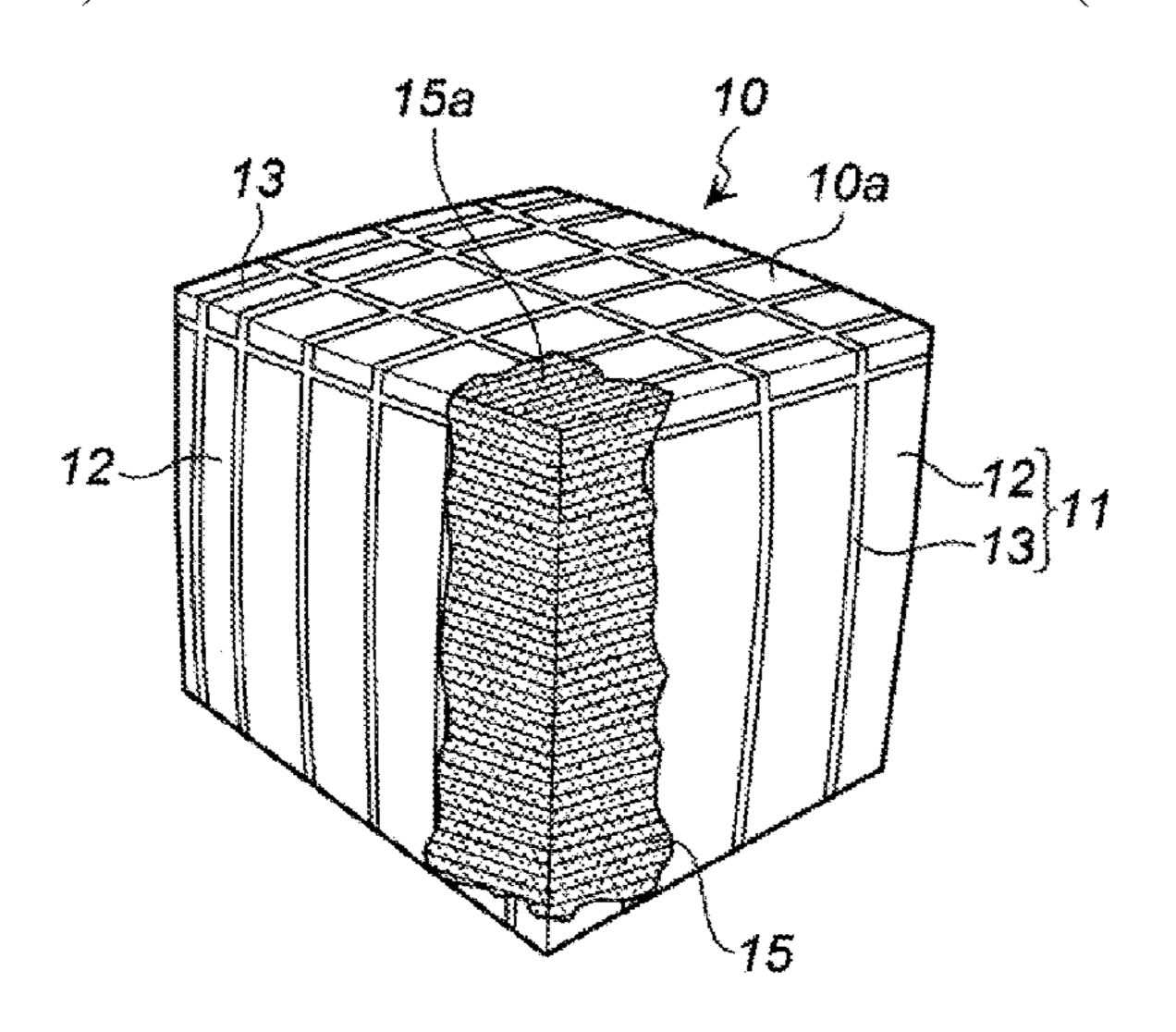
to 1,400 mm in length, 800 to 1,150 mm in width, and 800 to 1,100 mm in height, and a packing initial pressure between a top surface of the filter tow bale and the packing material is 6.3 kPa or less.
