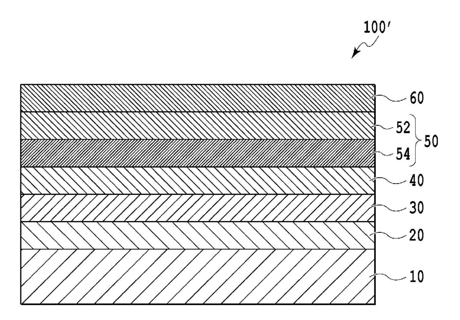
an FePt ordered alloy or an ordered alloy having Fe, Pt and Rh, and the second nonmagnetic crystal grain boundary includes carbon.
