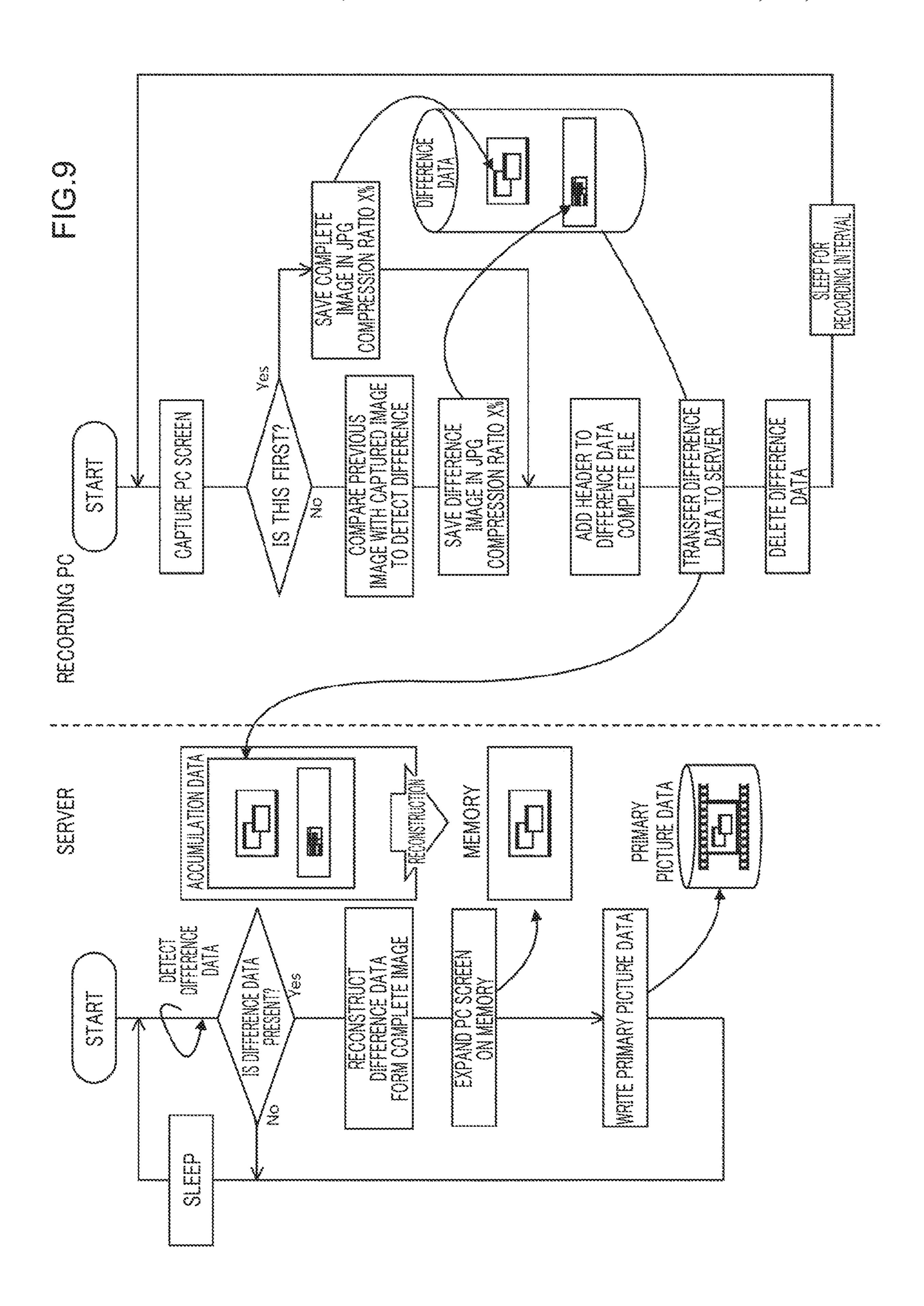
IMAGE COMPRESSING METHOD, IMAGE RECONSTRUCTING METHOD, IMAGE COMPRESSING DEVICE, IMAGE RECONSTRUCTING DEVICE, IMAGE COMPRESSING PROGRAM PRODUCT, AND IMAGE RECONSTRUCTING PROGRAM PRODUCT
