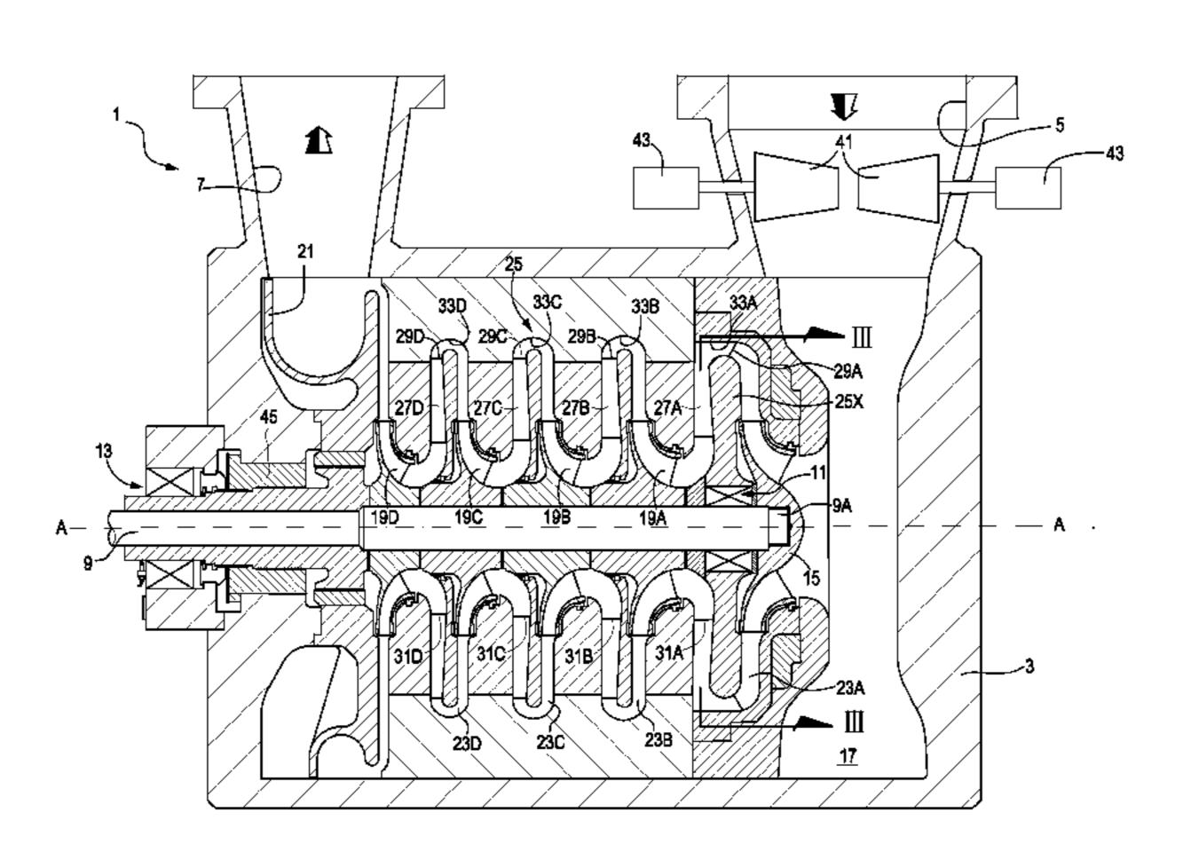
first diaphragm arrangement houses one of the first bearing and second bearing.
