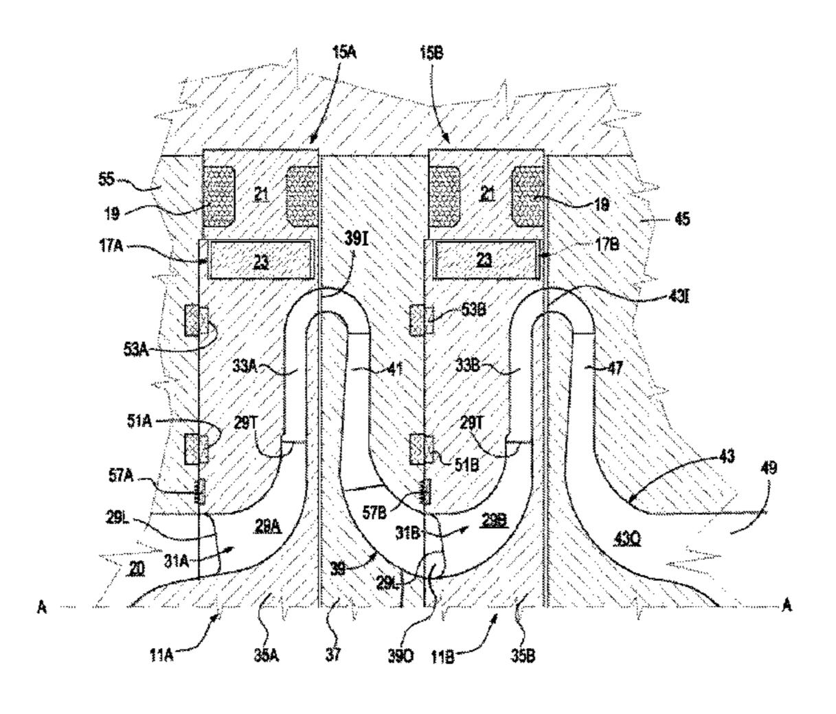
integral with the impeller. The motor rotor of each stage is arranged inside the respective motor stator.
