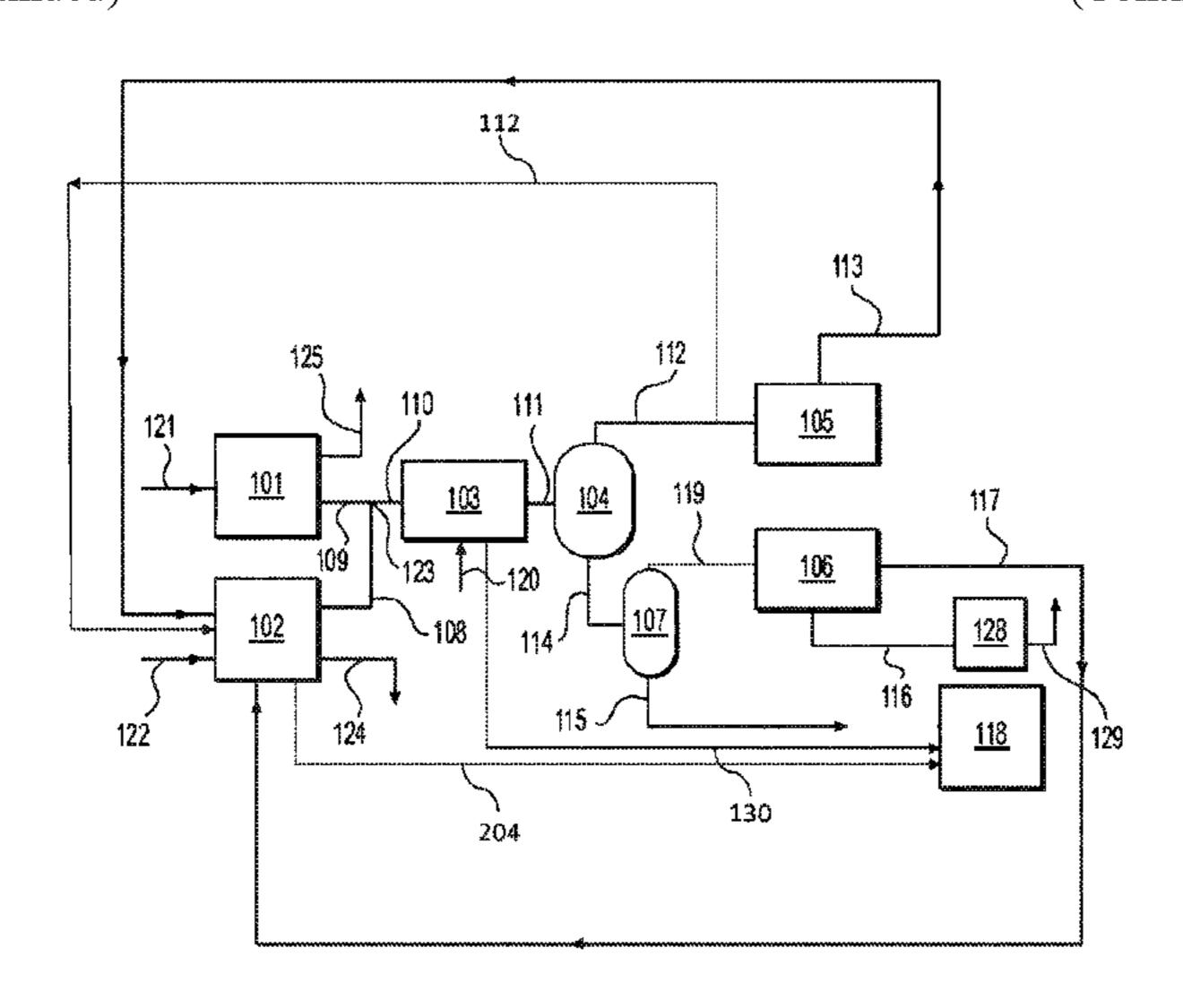
processing the combined stream to form a hydro-processed combined stream splitting the hydro-processed combined stream into a  $C_5/C_6$  stream, and a first aromatic rich stream, splitting the first aromatic rich stream into a second aromatic rich stream and a heavy oil stream.
